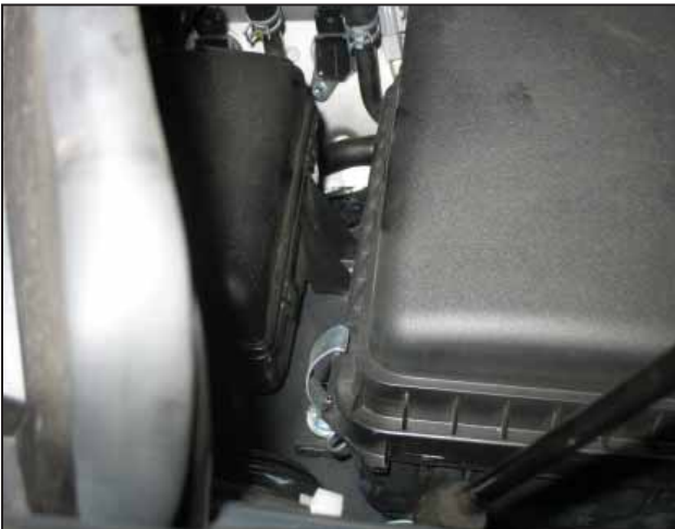
g . Unclip the third airbox clip.
