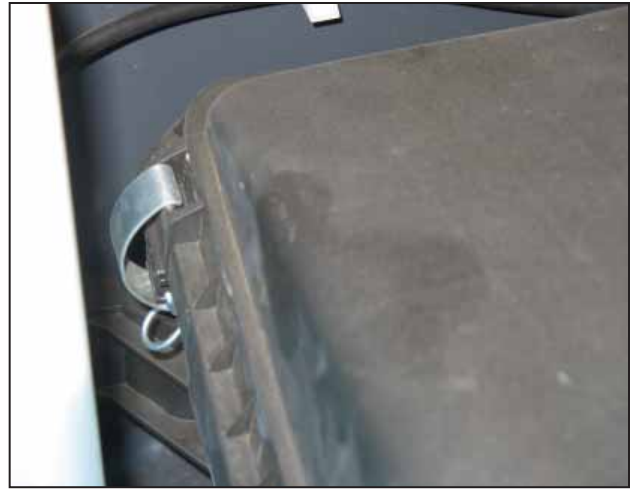
f. Unclip the second airbox clip.
