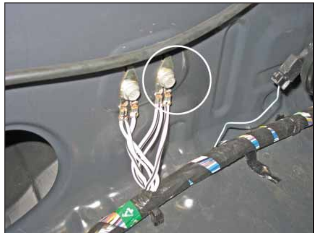
p. Within the engine bay, locate the ground bolt located on the passenger side inner fender. Remove the ground bolt closest to the firewall.
