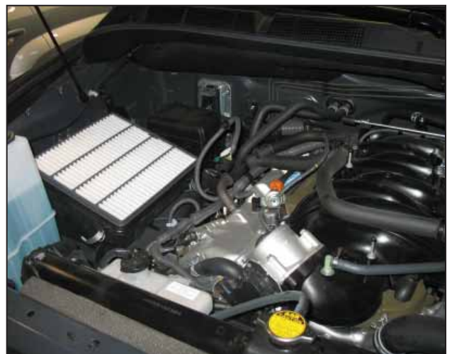
j. Remove the stock inlet tube and airbox lid assembly.
