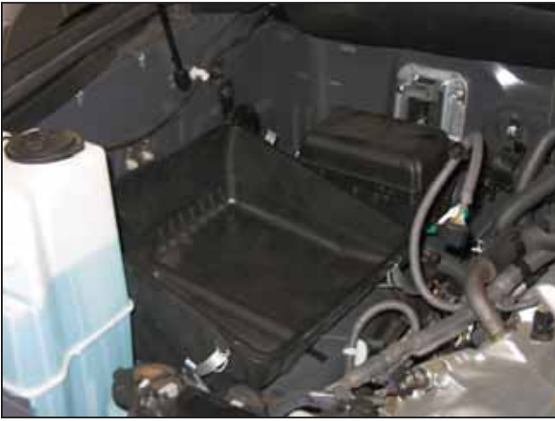
k. Remove the stock air filter from the lower airbox. box.
