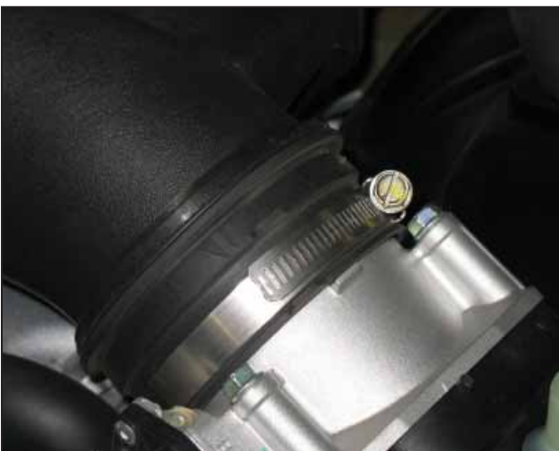
i. Loosen the hose clamp securing the stock inlet tube to the throttle body.
