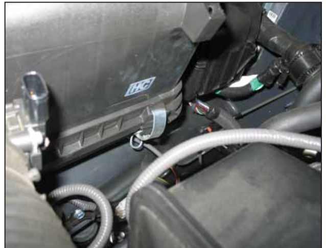
h. Unclip the fourth airbox clip.
