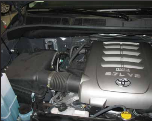
a. Factory airbox system installed.
