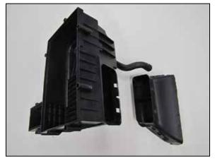
9. Remove the fresh air duct from the factory air filter housing.
