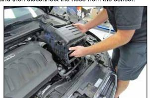
7. Pull up the air filter housing to remove it from the vehicle.
