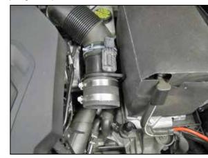
15. Install the provided coupler (08440) onto the mass air sensor and secure with the provided hose clamp.
