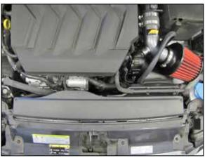
18. Reinstall the upper fresh air duct and secure with the factory hardware.
