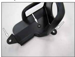
11. Install the three provided mounting grommets into the heat shield where shown.
