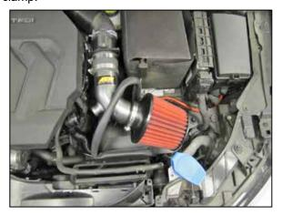
16. Install the AEM® intake kit so the grommets align with the mounting studs, connect the mass air sensor to the intake tube. Adjust the intake tube and filter for best fit and secure with the provided hardware and clamps.
