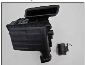
8. Remove the mass air sensor from the factory air filter housing.
