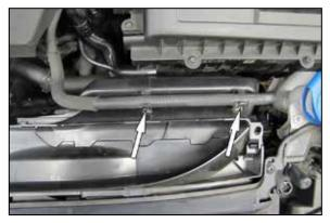
5. Unclip and move the coolant hose attached to the lower fresh air duct. Unclip and remove the lower fresh air duct from the vehicle.
