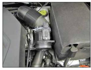
14. Reinstall the factory mass air sensor onto the factory intake tube and secure with the factory spring clamp.
