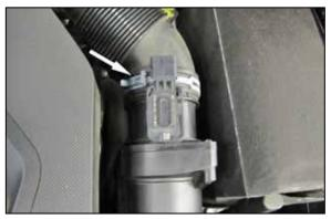
6. Release the spring clamp that secures the factory intake tube to the mass air sensor housing and then disconnect the hose from the sensor.
