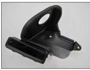
12. Install the factory fresh air duct into the heat shield as shown.
