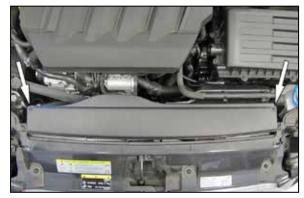
4. Remove the screws that secure the top of the fresh air duct and then remove the top from the vehicle.
