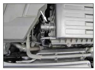
3. Disconnect the air injection hose from the upper air filter housing.
