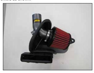
13. Install the rubber mounted stud into the heat shield and secure with the provided hardware. Install the AEM® intake tube into the heat shield and secure to the rubber mounted stud with the provided hardware. Install the AEM® air filter onto the intake tube and secure with the provided hose clamp.
