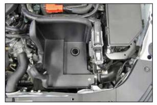
10. Install the heat shield assembly onto the mounting studs and secure with the provided hardware.
