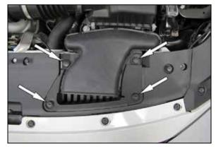
4. Remove the push pins that secure the fresh air duct and then remove the fresh air duct from the vehicle.
