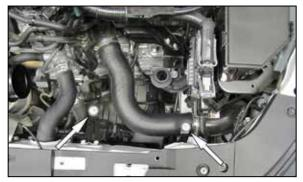
9. Install the two-provided rubber mounted studs onto the filter housing mounting locations.
