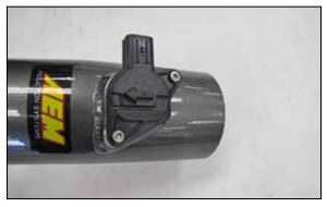
12. Remove the mass air sensor from the factory air filter housing and then install it into the AEM<sup>®</sup> intake tube and secure with the provided hardware.
