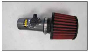
13. Install the AEM<sup>®</sup> air filter onto the intake tube and secure with the provided hose clamp.
