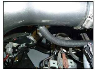
23. Connect the open end of the crank case vent hose to the fitting on the  $AEM^{\circledast}$  intake tube.
