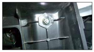
6. Release the air filter housing clips and remove the housing half and factory air filter. Remove the air filter housing retaining nut.
