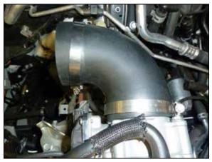
14. Install the provided 90° coupler onto the throttle body but do not completely tighten the hose clamp at this time.
