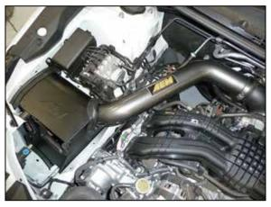
16. Install the intake assembly so the intake tube goes into the coupler at the throttle body and the heat shield rests on the frame and the mounting holes line up correctly.
