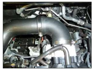
20. Align the intake tube for best fit and then secure the coupler hose clamp
