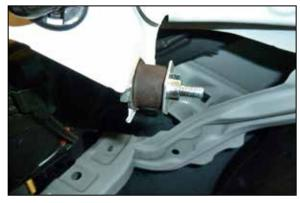
8. Remove the factory air filter housing mounting stud.
