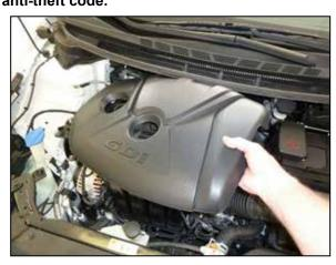
2. Lift the decorative engine cover up and remove it from the vehicle
