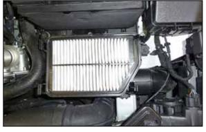
5. Remove the three bolts that secure the lower air filter housing to the inner fender and then remove the lower air filter housing from the vehicle. NOTE: AEM recommends that customers do not discard factory air intake.
