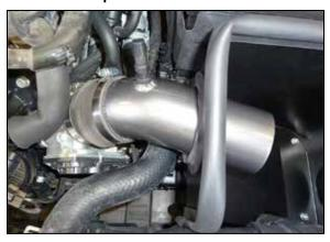
12. Install the AEM® tube through the heat shield and then into the coupler at the throttle body. Do not secure at this time.
