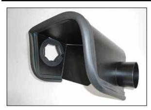
7. Install the 12" edge trim into the hole of the heat shield and the 34" section around the outside of the heat shield as shown.
