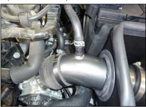
14. Connect the factory crank case vent hose to the fitting installed into the intake tube and secure with the factory clamp.
