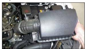
4. Loosen the hose clamp that secures the intake tube to the throttle body, release the two clips that secure the upper air filter housing and then remove the upper air filter housing and intake tube assembly.
