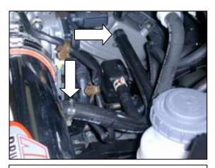
i. Install the supplied ½" breather hose between the intake pipe and the valve cover as shown. Use the supplied 1" hose clamps to secure. Secure the TBM wire harness to the valve cover breather hose using the supplied zip tie.
