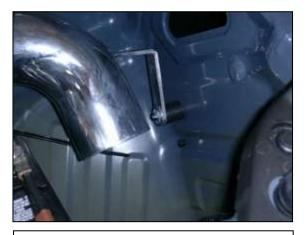
g. Guide the bracket on the intake pipe over the stud on the rubber mount. Once aligned, install the supplied washer and nylok nut onto the stud. Do not tighten until fitment is complete.
