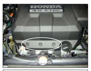
b. Remove the plastic intake air duct by removing the three plastic retaining clips. Be sure not to lose or damage any of these parts as they will be reinstalled.
