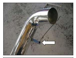
c. Check to see that the inside of the inlet pipe and air filter are clean and free from any foreign objects and/or obstructions. Install the supplied push in zip tie in the bracket as shown.
