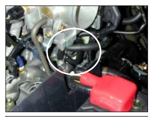
b. Install the provided 5/16" hose where the factory coolant line was removed. Use the supplied 3/4" hose clamps to secure the hose.
