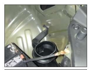
g. Remove the remaining bolt securing the air box to the chassis. Carefully remove the air box from the vehicle by lifting it straight up off the lower inlet tube.
