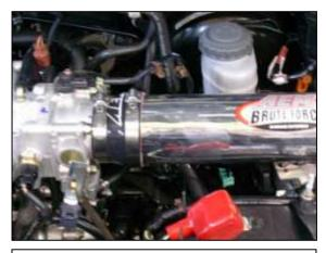
f. Install the AEM<sup>®</sup> intake pipe into the previously installed coupler.
