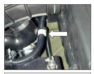
e. Unclip the wiring harness from the inlet air hose.
