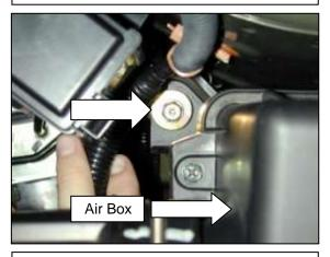
d. Remove the rear mounting bolt holding the stock air box in place.
