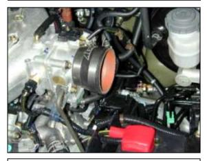
e. Install the silicone reinforced adapter over the throttle body and secure using a # 48 hose clamp.
