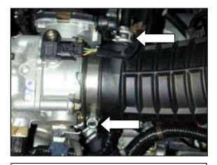
f. Loosen the hose clamp on the throttle body. Remove the valve cover breather hose from the air inlet pipe by compressing the flanges on the retaining clip and sliding the hose out.
