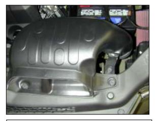
k. Install the stock air inlet duct using the three plastic connectors previously removed.
