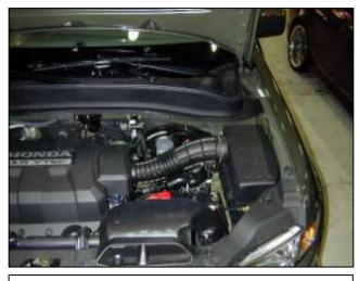
Stock air box system installed
