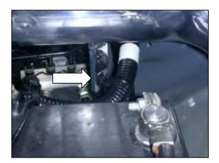
j. Secure the battery wiring harness to the intake pipe using the previously installed zip tie.
