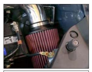
h. Install the AEM<sup>®</sup> air filter on to the end of the inlet tube. Push the air filter over the inlet pipe until the stop in the air filter is reached. Once proper fitment is achieved, install the supplied hose clamp to secure the filter onto the inlet pipe.
