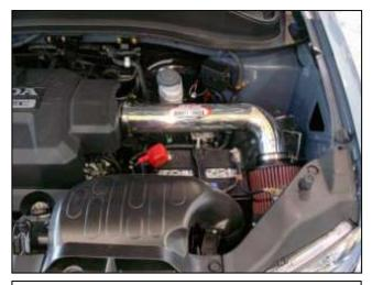
AEM<sup>®</sup> intake system installed
