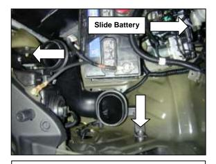
h. Remove the two bolts securing the lower inlet tube to the truck body. In order to remove the tube, loosen the battery hold down brackets and slide the battery forward for clearance. Once the inlet tube is removed, move the battery back to its original location and secure.
