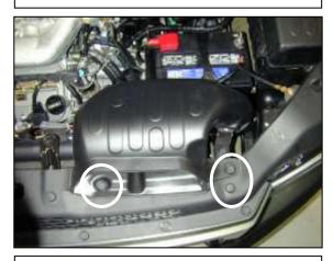
c. Remove the plastic intake air duct by removing the three plastic retaining clips. Be sure not to lose or damage any of these parts, they will be reused in installation.
