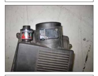
h. Remove the factory air filter restirction gauge from the stock air filter housing.
