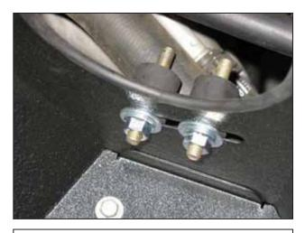
g. Install the two supplied rubber mounts into the slot on the heat shield. Secure each rubber mount with a washer and M8 nut. Secure the mounts with just enough slack for the mounts to slide in the slot.
