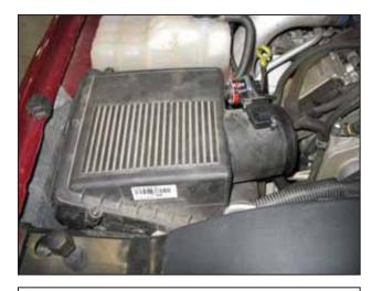
e. The air filter housing is held in place by two grommets on the mounting plate. Gently lift up on the air filter housing and remove it from the engine bay.
