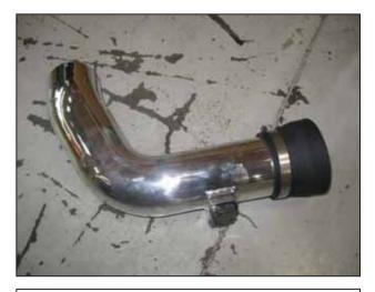
c. Install the previously removed MAF sensor into the upper intake pipe using the two supplied 8-32 bolts. Install the reducing coupler and #56 hose clamp onto the straight side of the upper intake pipe.
