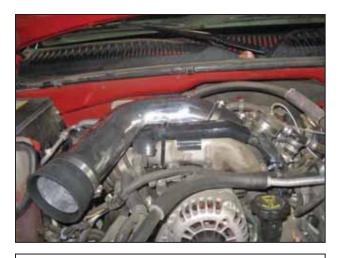
f. Install the upper intake pipe into the coupler on the turbo inlet. Slide the reducing coupler completely onto the intake pipe to allow room for the lower intake pipe to be positioned.
