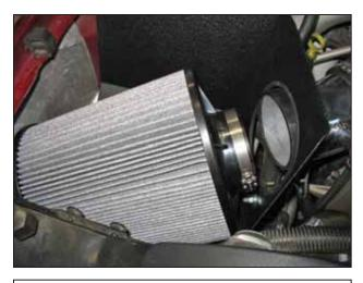
j. Lower the air filter into the heat sheild bay with the filter neck facing the engine. This will ease installation, as the air filter cannot easily be installed if the lower intake pipe is already installed.
