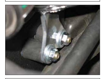
I. Slide the lower pipe and reducing coupler down the upper pipe until mounting bracket face is flush with the rubber mounts. Install the remaining M8 washers and nuts to secure the lower pipe's mounting bracket.
