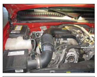
a. Factory air box system installed.
