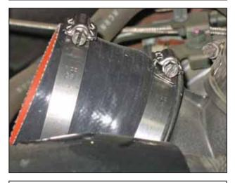
e. Install the straight coupler onto the turbo inlet hose and secure using two supplied #56 hose clamps as shown.
