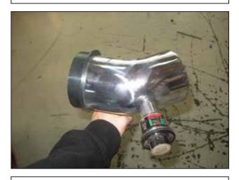
i. Install the previously removed air filter restriction gauge into the grommet installed in previous step. Also install the rubber filter adapter onto the filter end of the lower intake pipe.
