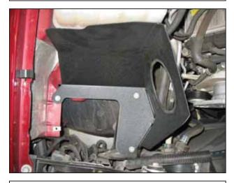
d. Install the heat shield in the engine bay aligning the holes with the moutning plate bolt locations. Secure it using three of the bolts removed during step 2f.
