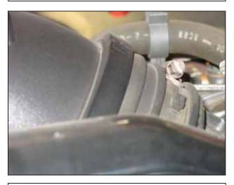
c. Lift up on the intake resonator to pop it off the mount and gain access to the hose clamp on the inlet tube. Loosen the hose clamps on both ends of the inlet tube.
