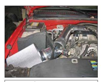
AEM® intake system installed
