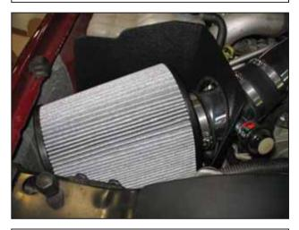
m. Slide the hose clamp onto the air filter's neck and attach the air filter assembly onto the filter adapter. Ensure the air filter is completely seated onto the adapter and the hose clamp is aligned with the filter adapter's lip. Once the hose clamp is properly aligned, secure the hose clamp, ensuring the filter neck's tabs compress and engage the filter adapter. Ensure the air filter does not make contact with any part of the vehicle and has adequate clearance.
