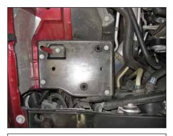
f. Remove the mounting plate for the air filter housing by removing the five bolts that secure it.
