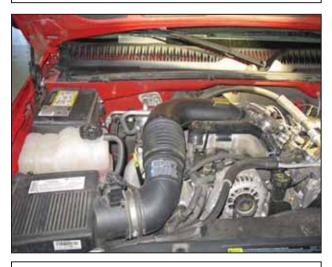
Factory air box system installed
