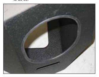
b. Install the supplied rubber edge trim onto the edge of the hole in the heat shield. Trim to fit.
