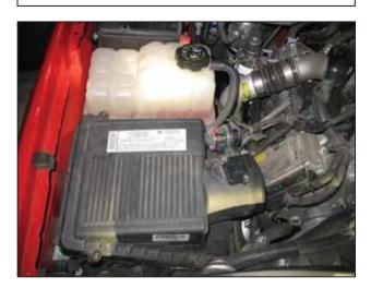
d. Remove the inlet tube and resonator from the engine bay.
