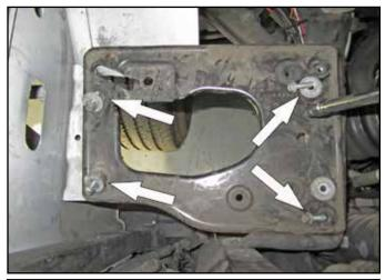
d. Using a 10mm socket, remove the four bolts retaining the stock air box mounting plate. Remove the mounting plate.
