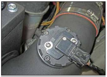
b. Install the mass air sensor on the mass air sensor adapter plate using the two buttonhead allen bolts provided.
