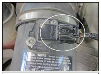
a. Depress the locking tab on the mass air sensor, then disconnect the mass air sensor.
