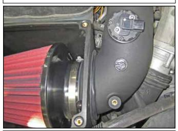
n. Loosely Install the 9-0427 lower intake tube through the bulb seal and into the air filter assembly as shown.
