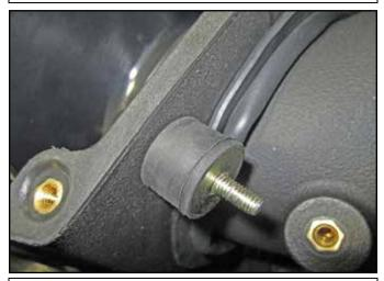
r. Install the 1228598 rubber isolator stud mount into the 6mm insert on the side of the airbox as shown. Tighten by hand.
