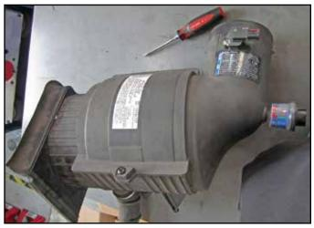
c. Pull up firmly on the stock air box starting on the side closest to the engine to dislodge it from the mounting grommets. Remove the air box from the engine bay.
