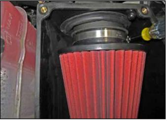
p. Fully seat the AEM® air filter onto the lower intake tube inlet and align it vertically as shown. Tighten the hose clamp at the air filter base.
