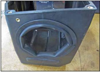
e. Install the bulb seal around the inside of the outlet hole on the 9-0406 air box as shown. Trim excess as needed.
