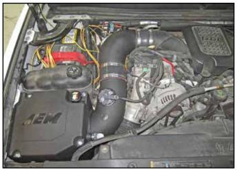
AEM® intake system installed.
