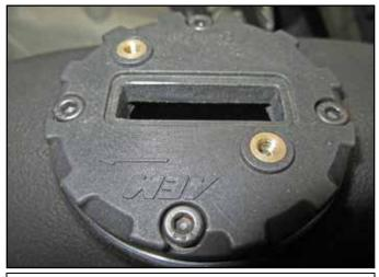
a. Install the mass air sensor adapter plate and O-ring seal in the 9-0427 lower intake tube using the four 4mm allen bolts provided.
