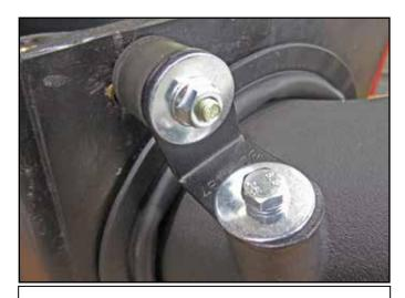
t. Install one flat washer, the split washer, and the M6 X 12mm hex bolt through the "L" bracket slot and into the mounting boss in the 9-0427 lower intake tube. Tighten the bolt and hex nut with a 10mm socket.
