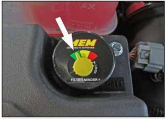
ab. Ensure the AEM® air filter minder gauge needle is pointing the green sector for the new AEM® Air Filter. Once the air filter is very dirty and the pressure drop (restriction) across it reaches 20 (inches of H20) the gauge needle will point to the red sector. This will mean it is time to wash the re-usable AEM® air filter.
