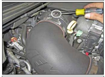
w. Fully seat the silicone hose at the engine intake port and tighten the hose clamp.
