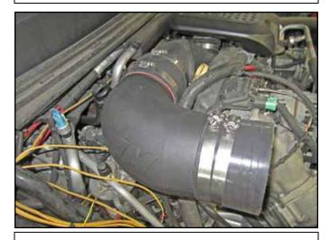
d. Install a #9472 hose clamp over the outlet hose and install the intake tube assembly onto the engine intake port as shown. Do not fully tighten the hose clamp.
