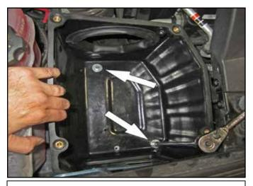
h. While pulling the air box toward the stock coolant reservoir to align the air box, install two M6 X 25mm bolts with two flat washers at the two mounting holes shown. Ensure the air box inlet window is aligned with the stock air inlet window in the sheet metal fender liner. Tighten the two bolts.
