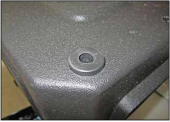
f. install the 784647 grommet into the larger left front mounting hole as shown.
