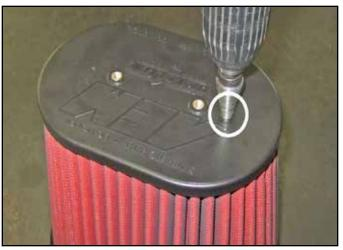
j. Drill a 1/4" diameter hole in the plastic cap of your new 21-2258DK AEM® Air Filter at the dimpled location as shown. **Clean out all plastic shavings from the inside of the air filter.**
