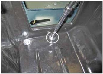
i. Install a M6 X 25mm bolt with a flat washer in the remaining mounting hole near the inlet window and thighten the bolt. Note that the large air inlet window is aligned with the smaller stock air inlet window in the vehicle fender.
