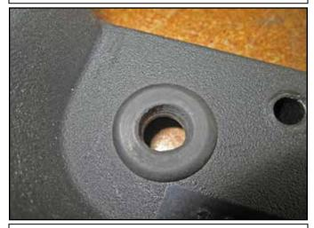
x. Install the 784642 grommet into the 3/4" hole in the corner of the 9-0411 air box lid as shown.
