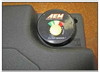
y. Install the 35-80321 air filter minder gauge into the large grommet. Use glass cleaner to lubricate the hole in the grommet if needed.
