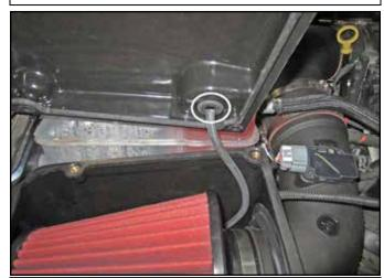
z. Mount the loose end of the 5/32" hose already at tached to the air filter cap onto the small port on the air filter minder gauge under the air box lid as shown.
