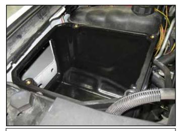
g. Place the air box into the engine bay into the stock location as shown. Ensure the new left front mount ing grommet is lined up with the threaded hole in the engine bay.
