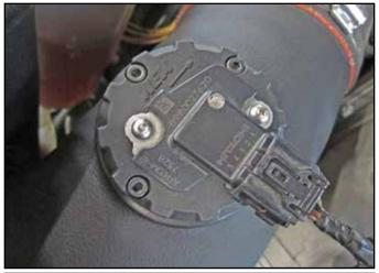
o. Re-connect the mass air sensor, fully seating the connector to lock it.
