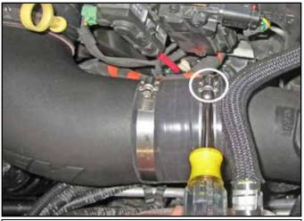
v. Tighten the hose clamp at the silicone hose connecting the upper and lower intake tubes.
