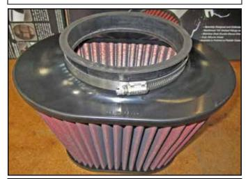
I. Install the large hose clamp provided onto the 21-2258DK AEM® DRYFLOW® Air Filter; then, Install the 5-2279 air filter base adapter into the outlet of the AEM® DRYFLOW® Air Filter.
