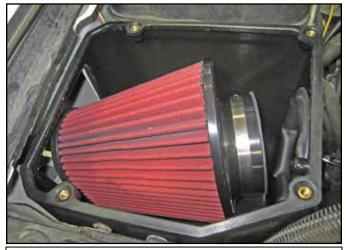
m. Place the AEM® Air Filter assembly into the air box as shown.
