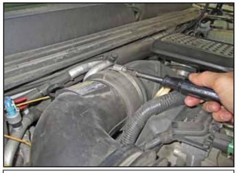
b. Loosen the two hose clamps retaining the stock intake tube, then remove the stock intake tube from the air box and the engine intake port.
