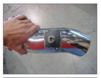
f. Install the IAT sensor into the grommet on the adapter plate as shown.
