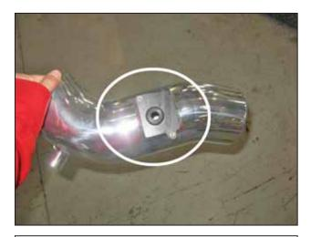
e. On vehicles with an IAT sensor, install provided adapter plate onto the intake pipe using the two supplied bolts. Install the supplied grommet into the plate.
