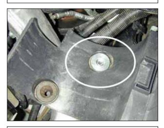
h. Install the billet aluminum stand into the rear rubber mount where the factory air box was removed.
