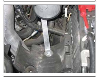
j. Install the supplied M6 washer and bolt through the bottom of the aluminum stand. Secure the bolt using another M6 washer and serrated nut as illustrated in step 3k.
