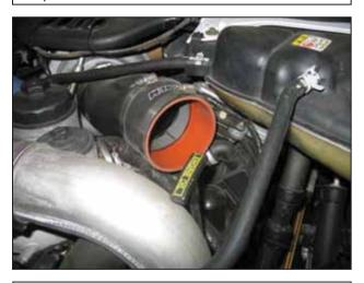
g. Install the silicone coupler onto the turbo inlet and secure using two #64 hose clamps.
