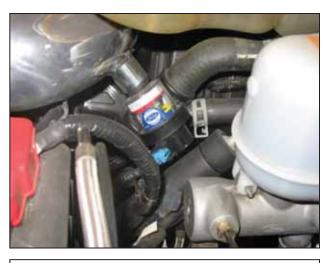
p. Plug the air filter restriction gauge into the wiring harness. Ensure the wiring harness will not make contact with any components that will get HOT.
