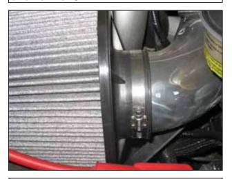
m. Slide the hose clamp onto the air filter's neck and attach the air filter assembly onto the filter adapter. Ensure the air filter is completely seated onto the adapter and the hose clamp is aligned with the filter adapter's lip. Once the hose clamp is properly aligned, secure the hose clamp, ensuring the filter neck's tabs compress and engage.
