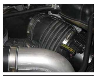
b. Loosen the hose clamps securing the flexible inlet hose between the turbo inlet and the air filter housing. Remove the hose.
