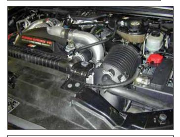
Factory air box system installed
