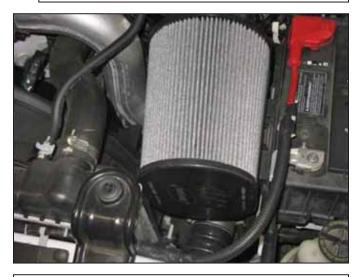
AEM<sup>®</sup> intake system installed
