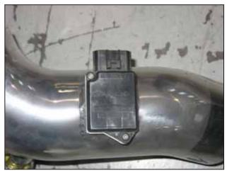
d. On vehicles with a MAF sensor, install the sensor into the intake pipe using the two factory bolts removed in step 2f). If your vehicle is equipped with an IAT, skip to step 3e).
