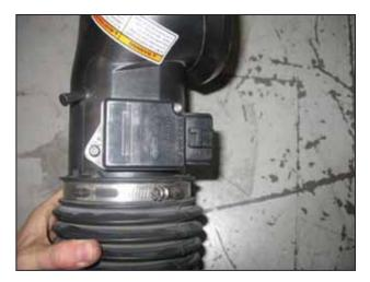
f. Remove the factory IAT sensor or MAF sensor from the stock air filter housing.
