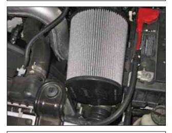
n. Ensure the air filter does not make contact with any part of the vehicle and has adequate clearance.
