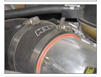
i. Install the intake pipe into the coupler on the turbo inlet. Align the intake pipe mounting bracket with the previously installed aluminum stand. Use a #64 hose clamp to secure.
