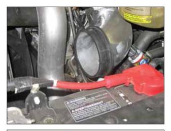
I. Install the supplied air filter adapter by stretching it over the filter end of the intake pipe.
