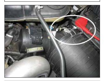
d. Unclasp the retaining clips holding the back side of the air filter housing together. Remove the rear side of the air filter housing by lifting up and pulling it out of the engine bay.
