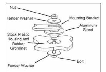
k. Diagram for mounting bracket. Once aligned properly, fully tighten the nut.
