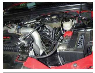
c. Factory air box system removed.
