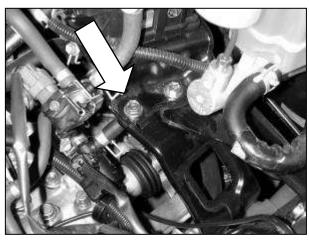
c. Remove the forward-most M8 bolt from the black bracket under the brake master cylinder.
