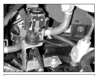
g. Use one of the supplied zip ties to secure the upper VSV to the bracket. Make sure the zip tie rests in the notches in the bracket to ensure that it does not slide off.
