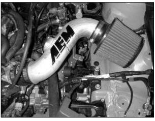
I. Install the throttle body end of the pipe into the silicone coupler. Plug in the MAF sensor on the back side of the pipe. **NOTE: Failure to plug the MAF sensor in will cause the check engine light to illuminate and the vehicle to run poorly.**
