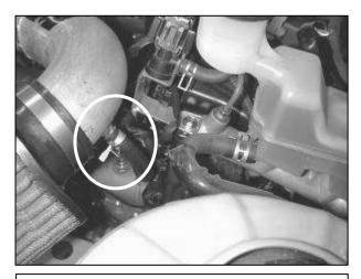
n. Use the other stock spring clamp on the intake pipe side of the 5/16" vacuum hose. Route the hose carefully to avoid kinks.
