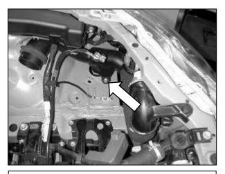
m. Remove the stock intake air duct from the engine bay. The duct is retained by one bolt and one plastic rivet. Pry the center of the plastic rivet up with a small screwdriver; the entire rivet should pull out.
