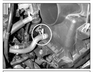
f. Remove the large vacuum line from the engine side of the air box lid.
