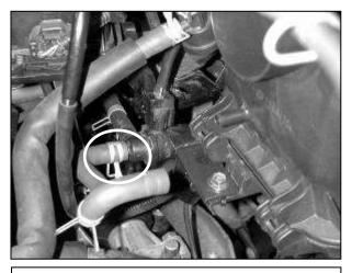
g. Remove the other side of the large vacuum line from the VSV mounted to the air box. Keep both vacuum line spring clamps; they will be reused with the  $AEM^{\textcircled{B}}$  intake system.
