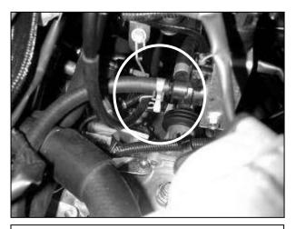
m. Replace the vacuum line removed in step 2g with the supplied length of 5/16" vacuum hose. Reuse the stock spring clamp.
