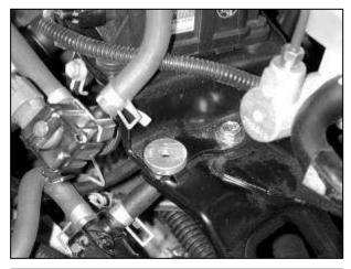
d. Place the supplied VSV bracket spacer inline with the hole exposed in the previous step.
