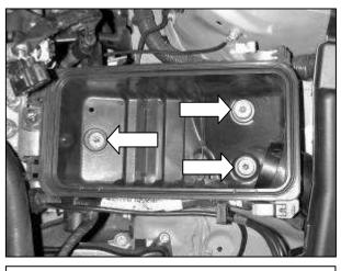
I. Remove the three bolts retaining the lower air box. Remove the lower air box from the vehicle.
