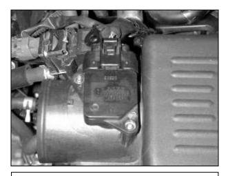
e. Remove the air flow meter connector from the sensor. Remove the two small screws and remove the sensor from the air box. Use care when removing this component, as it can be easily damaged. Set the air flow meter aside in a safe place.
