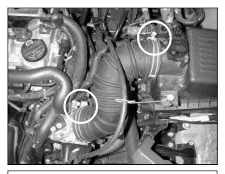
d. Loosen the two 10mm hose clamps at the throttle body and air box. Remove the stock rubber intake hose from the engine bay.
