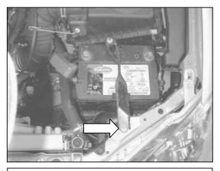
c. Disconnect the positive battery terminal. Remove the bolt on the radiator support that secures the battery bracket. Unhook the rod at the rear of the battery bracket. Remove the battery from the vehicle. **NOTE: Refer to the owner's manual for specific details regarding battery removal.**
