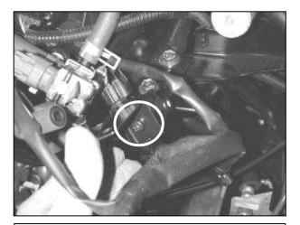
k. Remove the phillips head screw that secures the metal bracket to the VSV. This bracket will not be reused with the  $AEM^{\circledast}$  intake system.
