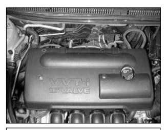
b. Remove the two nuts and two plastic rivets that hold the plastic engine cover on. The plastic rivets may be gently lifted with a small screwdriver. Remove the engine cover.
