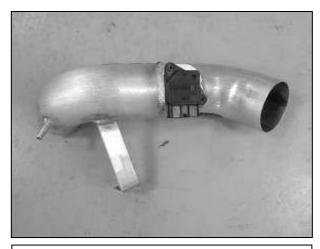
h. Mount the MAF sensor to the adaptor on the underside of the  $AEM^{\textcircled{B}}$  intake pipe using the two supplied 8-32 cap screws.
