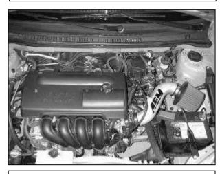
AEM<sup>®</sup> intake system installed
