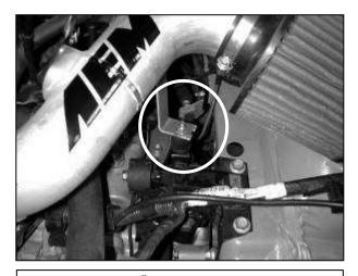
k. Install the AEM<sup>®</sup> intake pipe into the engine bay with the air filter already installed. The intake bracket should line up with the rubber mount. Loosely secure the bracket to the rubber mount with the supplied M6 washer and lock nut. Refer to the diagram above for proper rubber mount installation.
