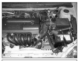
Factory air box system installed
