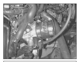
i. Place the supplied silicone hose on the throttle body. Loosely secure the hose with the two supplied 2.75" hose clamps.
