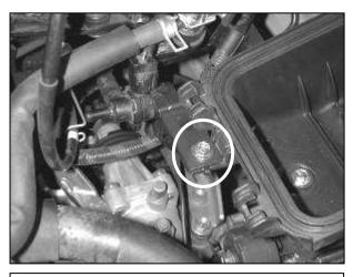
j. Remove the bolt holding the lower VSV bracket to the air box.
