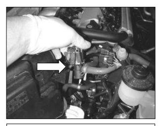
h. Release the two air box cover clips and lift the air box cover to gain access to the VSV with the blue connector on the back side of the cover. Press the tab on the VSV and slide upwards to release the VSV from the air box cover.
