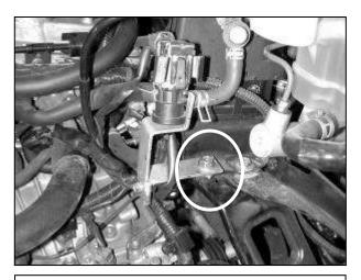
f. Use the supplied M8 bolt to secure the assembly to the bracket beneath the master cylinder. Be sure that the spacer remains in place. Rest the upper VSV on the bracket as shown. The rear vacuum line may need to be pulled back slightly to clear the bracket.
