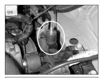
j. Install the supplied rubber mount onto the metal lower air box bracket. See diagram below for proper rubber mount installation.
