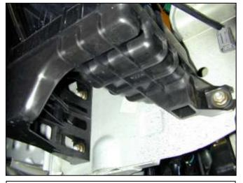
I. Release the three nuts securing the resonator box. Remove the resonator box from the vehicle.
