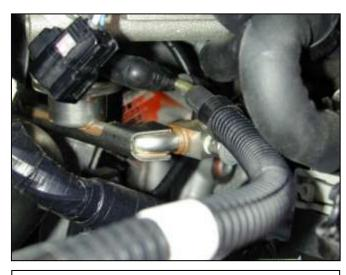
c. Follow the vacuum hose up to the 'T fitting. Pull the vacuum hose off of the 'T' fitting. Remove the hose from the vehicle.
