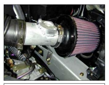
g. Insert other end of pipe into the stock inlet hose. Place mounting tab under the bolt in the frame rail.
