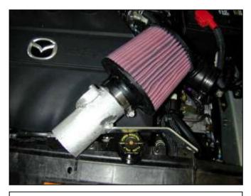
f. Install the air filter onto the end of the pipe as shown.
