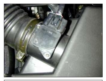
b. Unplug MAF sensor and loosen hose clamp at air box inlet.
