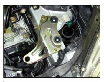
g. Pull the air box up and out of the engine bay. Remove the two bolts holding down the air box bracket and remove the bracket from the vehicle.
