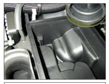
f. Pull vacuum hose off of the nipple on the air box.
