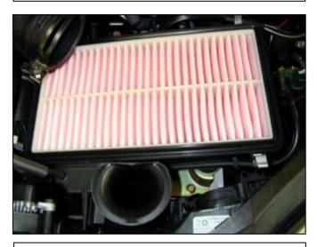
d. Remove the air filter from the lower air box.
