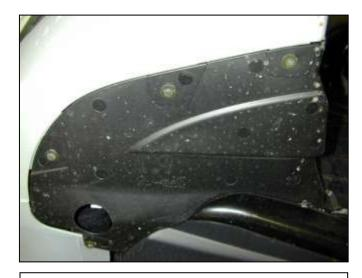
j. Remove the four screws on the bottom of the fender liner.
