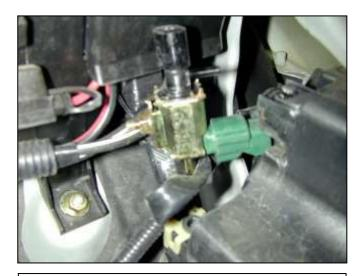
h. Remove the vacuum solenoid from the air box. Remove all vacuum lines from the solenoid. Plug green connector back into solenoid and secure it to a wiring harness utilizing the supplied zip tie.
