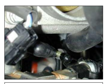
d. Install the supplied vacuum cap onto the open port on the 'T' fitting.
