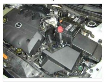
a. Stock air box system installed.
