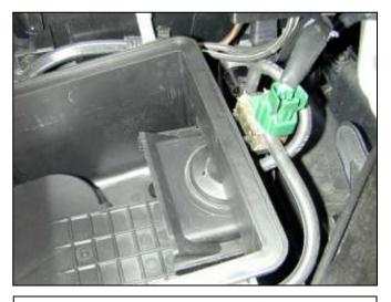
e. Unplug green connector on the vacuum solenoid.
