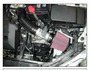
i. Check the clearance of the air filter with respect to the surrounding surfaces. Tighten the hose clamp on the inlet hose and the frame bolt.
