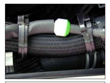
b. Release the two hose clamps that hold the vacuum hose to the radiator hose.
