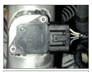
h. Install the air flow sensor into the inlet pipe utilizing the supplied screws. Plug in the air flow sensor.
