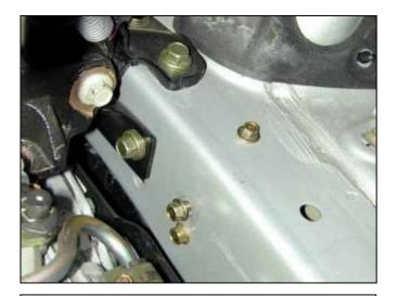
e. Loosen the upper bolt on the frame rail.
