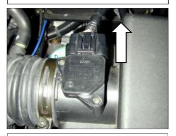
d. Unplug the mass air flow (MAF) sensor. Remove MAF sensor from air box.
