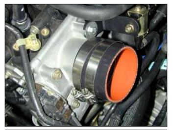
f. Install the supplied silicone hose onto throttle body.
