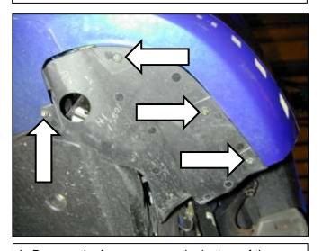
k. Remove the four screws on the bottom of the fender liner.
