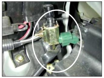
h. Remove the vacuum solenoid from the air box. Remove the 2 vacuum lines from the solenoid. **Plug the green connector back** into solenoid and secure it to a wiring harness utilizing the supplied zip tie.
