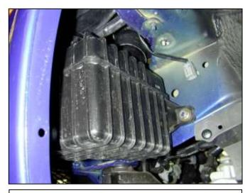
m. Remove the three nuts that secure the lower air box to the vehicle.
