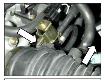
e. Pull the crankcase breather hose off of the inlet tubing. Remove the nut that secures the vacuum solenoid to the metal bracket and save it for later use.
