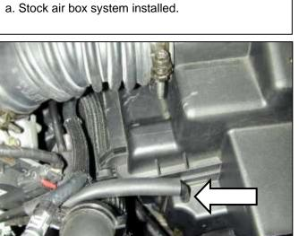
c. Pull the vacuum hose off of the air box nipple.
