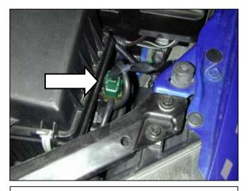
b. Release the green plug on the vacuum solenoid located next to the air box.
