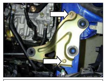
i. Remove the air box support plate.
