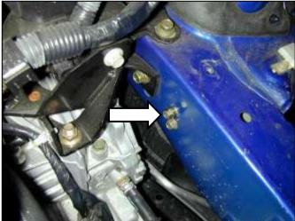
g. Remove the upper bolt in the frame rail.
