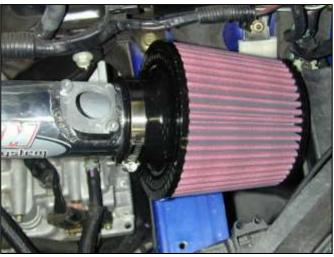
I. Install the air filter onto the end of the pipe.
