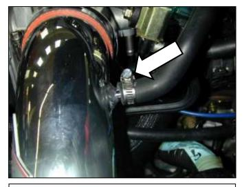
k. Install crankcase breather hose onto nipple. Secure hose with the supplied 3/4" hose clamp.
