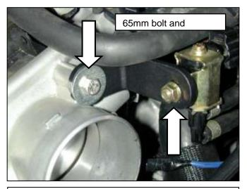
d. Remove the upper, rear bolt on the throttle body.
