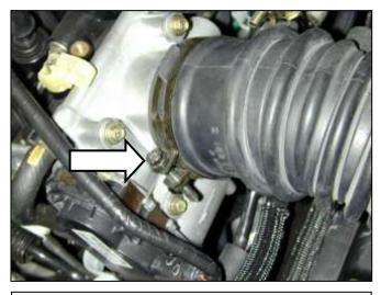
f. Loosen the hose clamp at the throttle body. Pull the inlet hose off of the throttle body.
