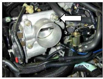
e. Use the supplied 65mm bolt and washer to secure the bracket to the throttle body. Install vacuum solenoid utilizing the stock nut as shown.
