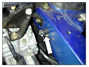
h. Install supplied rubber mount as shown.
