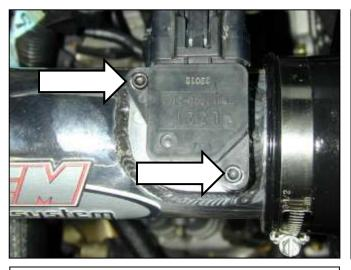
m. Install the MAF sensor into inlet pipe. Secure it with the supplied screws. Plug in the MAF sensor.
