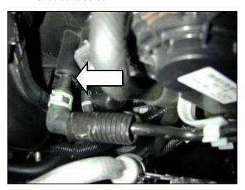
b. Follow the vacuum hose (that was earlier pulled off of the air box) up to the intake manifold. Pull vacuum hose off nipple on the intake manifold.
