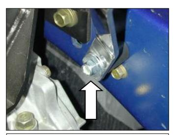
j. Place the support bracket behind the rubber mount washer as shown.
