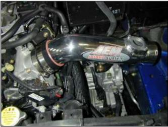
i. Install the inlet pipe as shown. Do not tighten hose clamps.
