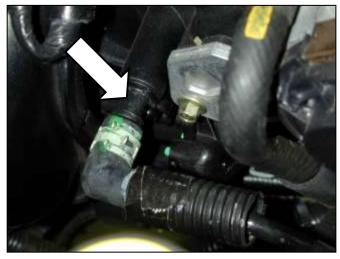
c. Cover the open nipple with the supplied vacuum cap.
