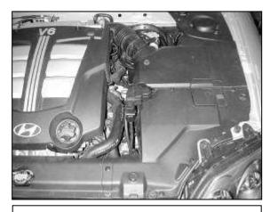
a. Remove the upper plastic cover covering the stock intake system.
