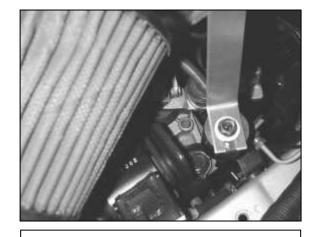
c. Remove the bolt securing the vibration dampener. Install the bracket securing it with the supplied bolt.
