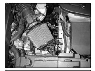
b. Install the filter over the air flow sensor and secure using the supplied hose clamp.
