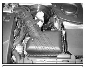
b. Remove the hose clamp securing the upper filter box to the air flow sensor. Unlatch the two clips securing the upper filter box and remove.
