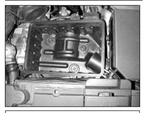
c. Remove the filter. Remove the three bolts securing the lower filter box and remove from vehicle.
