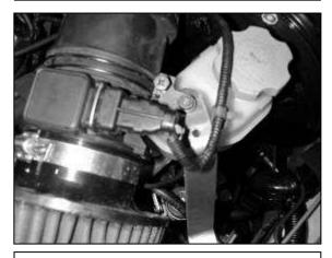
d. Remove the wire harness clip from the hose clamp. Install the bracket with the supplied bolt, washer and nut.
