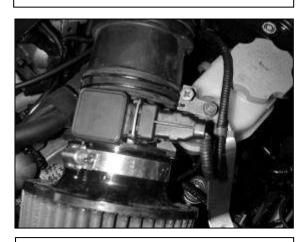
e. Install the wire harness clip into the second hole on the mounting bracket.
