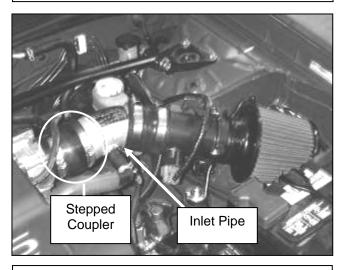
d. Attach stepped coupler to throttle body with provided hose clamps. Attach inlet pipe. Note hose clamp sizes are different.
