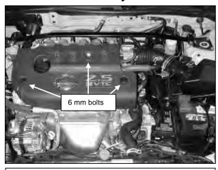
a. Loosen the three 6mm bolts on the engine cover and remove it.
