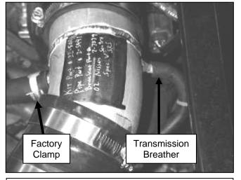
e. Attach factory crank case breather tube with factory clamp. Attach transmission breather hose to the fitting on the firewall side of the pipe. Manual transmission cars will have to attach the hose to the pipe if not, put the vacuum cap included in the kit on to the nipple.
