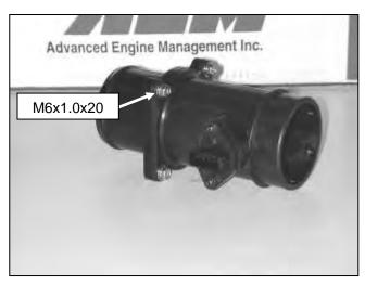
c. Install the included MAF adaptor onto the sensor using only 3 of the 4 factory bolts from step 3b. Install the M6x1.0x20 bolt in location specified in the image above.
