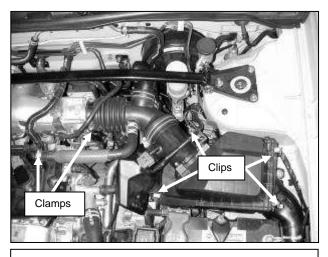
b. Loosen the air filter tube hose clamps, air cleaner lid clips and then remove the air filter lid and intake hose assembly.
