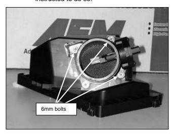
b. Loosen the four 6mm bolts, and remove the MAF sensor from the air cleaner lid.
