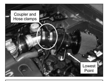
f. Attach the MAF assembly with the coupler and hose clamps. Make sure the M6x1.0x20 bolt is at the lowest point. The flow arrow on the MAF should point towards the throttle body. Attach the air filter assembly and secure.
