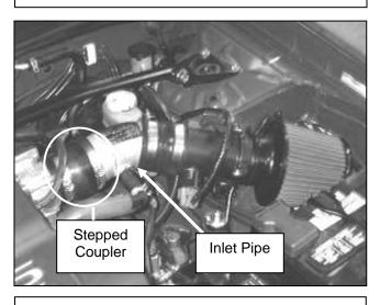
d. Attach stepped coupler to throttle body with provided hose clamps. Attach inlet pipe. Note hose clamp sizes are different.
