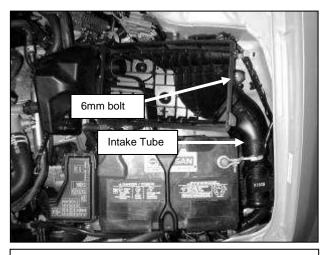
c. Loosen the 6mm air cleaner hold down bolt, and remove the air cleaner assembly and intake tube.
