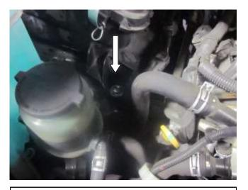
i. Make sure air box is sitting on the previously installed mount and install the washer (559960) and nut (444.460.04) and tighten. Also re-install and tighten the backside bolt that was removed in step 2e.
