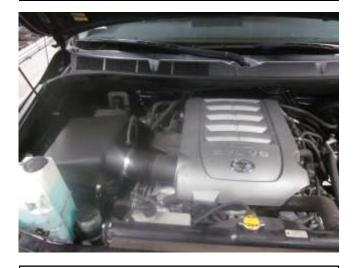
Factory air box system installed
