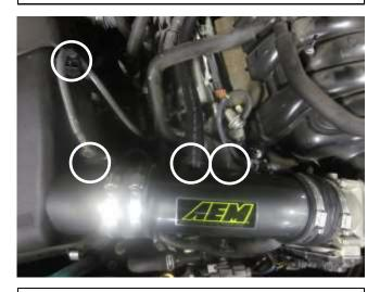
g. Re-clip the mass air flow sensor harness to the sensor. Re-attach the small vacuum line back onto the AEM intake tube. Install the provided hose (5-7022) onto the AEM intake tube.
