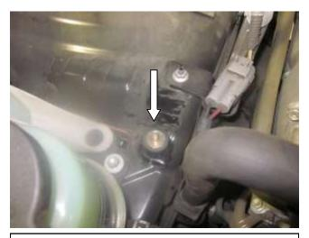
b. Install the provided (1228560) mount into the body of the vehicle where the M6 bolt was removed in 2e.
