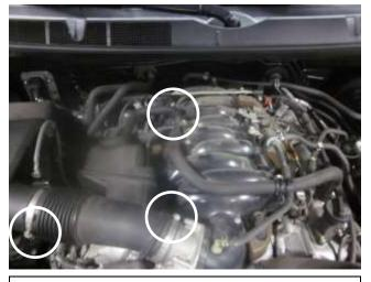
b. Loosen the hose clamp at the throttle body and the air box. Disconnect the small vacuum line on the intake resonator and the large vacuum line at the "T" above the intake manifold.
