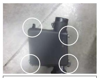
h. Unlatch the 4 clips holding the upper air box to the lower air box and remove the stock filter.
