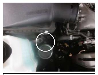
e. Loosen and remove the M6 bolts securing the air box to the vehicle. **Note:** One of the bolts is on the backside of the air box (not shown). One of the bolts will be reused.
