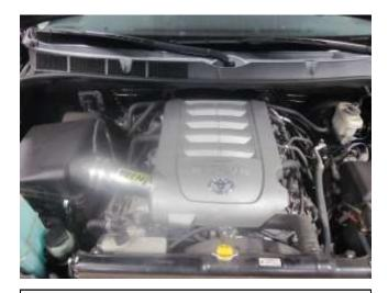
AEM<sup>®</sup> intake system installed
