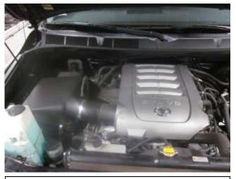
a. Remove the engine cover by pulling up and out.
