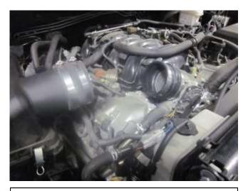
e. Slide the provided hose (5-1086) with the hose clamps (9456) onto the air box. Slide the provided hump hose (08657) with the hose clamps (9456 & 9452) over the throttle body.
