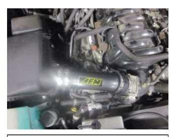
f. Lift the air box slightly and slide the AEM intake into the throttle body hose, then the air box hose while lowering the air box over the mount installed in 3b. Tighten all four hose clamps at this point.
