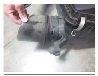
g. Disconnect the stock air inlet form the air box.
