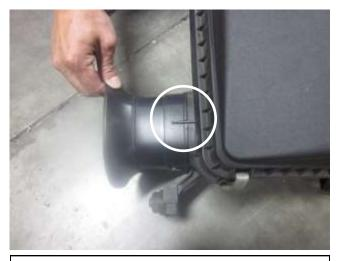
a. Install the AEM air accelerator onto the air box by aligning the slot in the box and the air horn.
