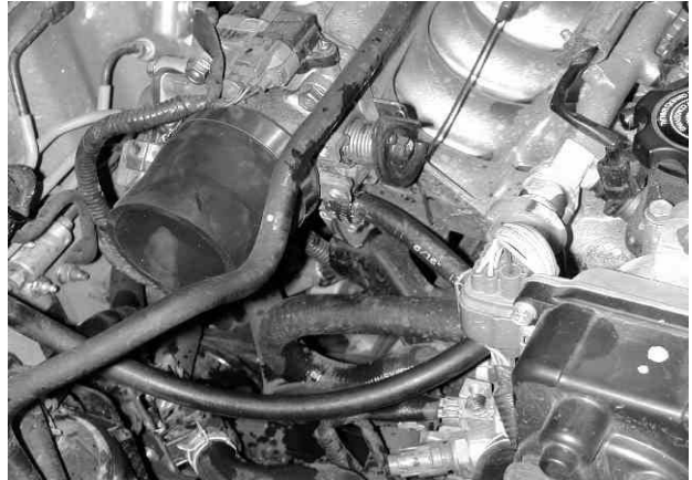
b) Insert the 2.5" x 3.0" coupler on to the throttle body (this is a tight fit). Slide the two #44 hose clamps over the end of the coupler.
