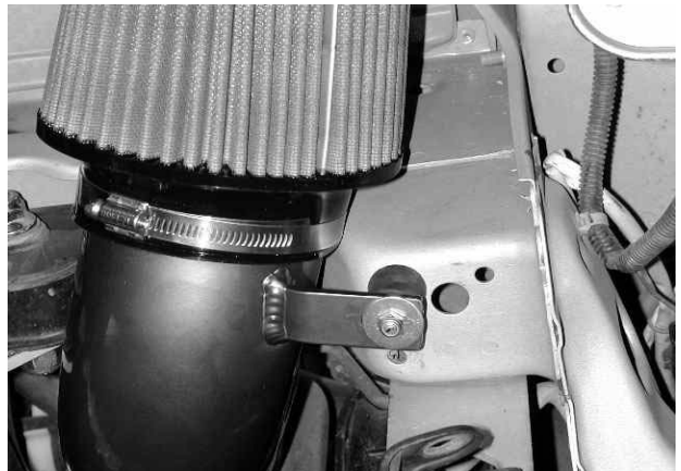
d) Align the tab on the intake pipe with the rubber mount. Install the 6mm nut and washer according to the diagram below. Do not tighten the nut.
