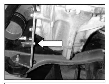
b. Install the supplied rubber mount using the included nylock nut and washer.
