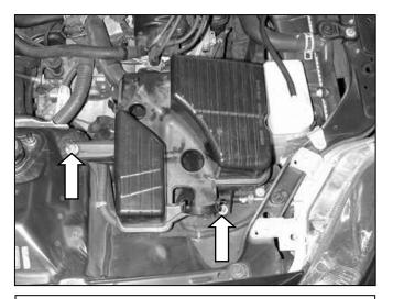
b. Loosen the bolts holding the resonator box to the frame rail, and remove it.
