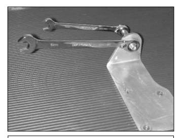
c. Install the factory mounting stud from step b on the supplied engine mount bracket, using the supplied Nylock nut and washer.
