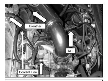
d. Using the supplied coupler and clamps, install the upper intake pipe. Install the intake air temp sensor, and the cam cover breather line onto the nipple, and secure it with the included clamp. Install the coolant line, and secure it with the included clamps.
