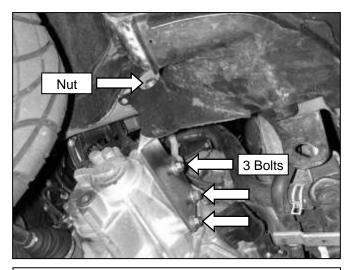
d. Using the supplied bolts and the factory washers, install the AEM<sup>®</sup> engine mount on the transmission, torque bolts to 61 ft-lb. Then replace the factory washer and nut on the mounting stud.
