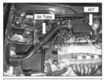
a. Remove the intake air temp sensor (IAT) from the air filter lid, then remove the air tube and filter lid from the vehicle.
