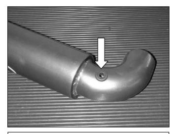
c. Install the rubber grommet in the 5/8" hole in the upper intake pipe.
