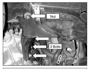
a. Remove the engine mount nut, then loosen the three bolts, and remove the mount.
