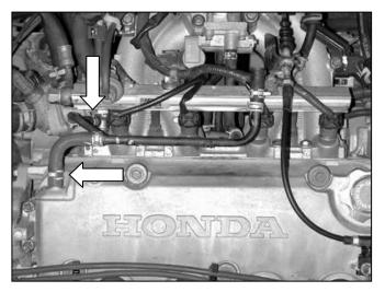
d. Remove the clamps as shown, and remove the metal breather pipe assembly.
