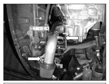
e. Install the lower intake pipe using the included coupler and hose clamps. Secure the bracket to the rubber mount using the supplied nylock nut and washer, as shown. Install the air filter and secure it with the supplied clamp.
