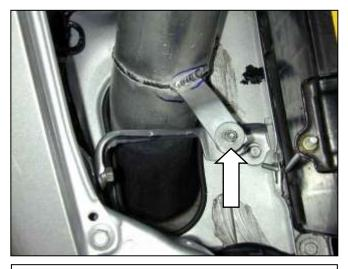
h. Install the washer and then the nylok nut on top of the intake bracket. Do not tighten the nut all the way down.
