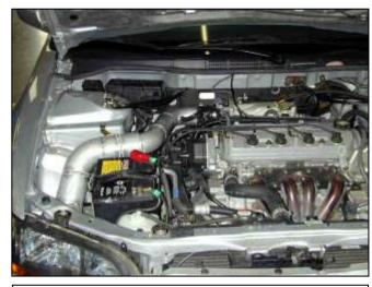
AEM® intake system installed
