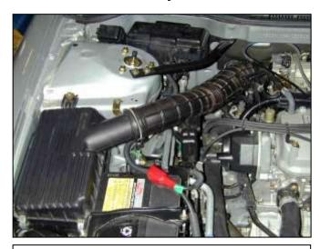
a. Factory air box system installed.
