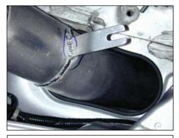
d. Slide the large diameter end of the AEM® intake pipe through the hole in the engine bay. Then slip the smaller end under the strut tower brace. Be sure to use rags to prevent the intake pipe from getting scratched.
