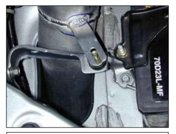
g. Install the air filter housing bracket in its original location with the rubber mount attached.
