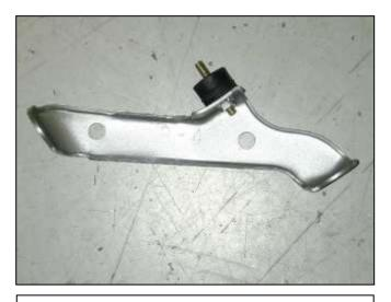
f. Using the previously removed stock air-filter housing bracket, thread the supplied rubber mount in the hole where the air-filter housing was bolted.
