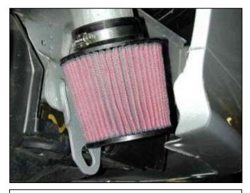
j. Install the AEM<sup>®</sup> air filter on to the end of the inlet tube. Push the air filter over the inlet pipe up to the stop in the filter. Install one hose clamp to secure the filter onto the inlet pipe. Once proper fitment is achieved, tighten the hose clamp.
