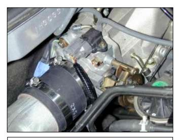
e. Place the reducer coupler over the throttle body but do not tighten the hose clamp completely.
