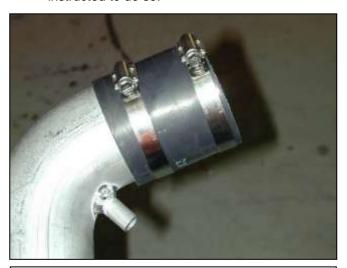
b. Ensure the inside of the AEM intake pipe and air filter are clean and free from any foreign objects and/or obstructions. Install the 2.50"-2.75" reinforced reducer over the throttle body end of the intake pipe using the 2.5" and 2.75" hose clamps as shown.
