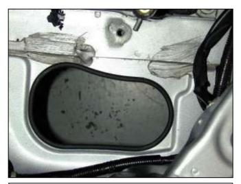
c. Install the rubber edge trim around the edge of the hole that passes through the engine bay. **NOTE: The edge trim will need to be cut to size.**
