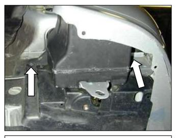
e. Remove the two bolts securing the resonator box. Pull the resonator box out from the bottom of the vehicle.
