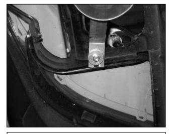
e. Slide the intake pipe support into place on the rubber mount and secure with a washer and lock nut as shown. Do not completely tighten.
