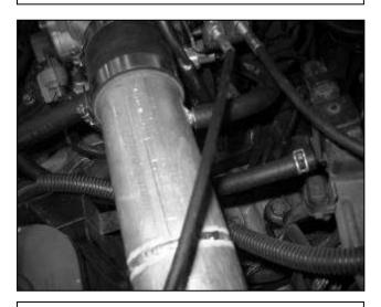
d. Slip the larger end of the intake pipe through the opening of the fender well, while sliding the smaller section of the intake pipe under the throttle cables and into the coupler attached to the throttle body. Push the pipe in until it stops.
