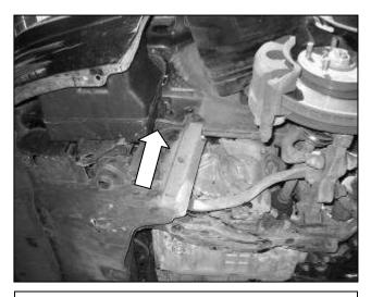
d. Remove the plastic clips holding the lower splash shield and fender liner on. Remove the two bolts holding the intake resonator in place, then lower the resonator out from the bottom of the vehicle.
