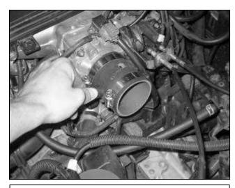
c. Install the 2.5" coupler onto the throttle body using the #40 hose clamps. Be sure that hose clamps are positioned on the opposite side of the throttle cables. Plug the breather hose into the inlet on the opposite side of the hex head plug.
