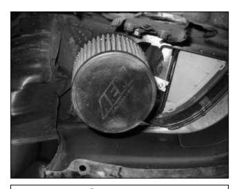
g. Install the AEM<sup>®</sup> air filter onto the end of the intake pipe. Push the air filter onto the intake pipe until the stop in the air filter is reached. Once proper fitment and clearance is achieved, secure the air filter to the intake pipe with the supplied hose clamp.
