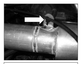
f. Attach the vacuum line to the inlet nipple of the intake pipe. Insert the plug side of the zip tie into the mounting tab of the intake pipe. Secure the throttle cable with the zip tie as shown and clip off the excess length of the zip-tie.
