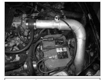
AEM® intake system installed
