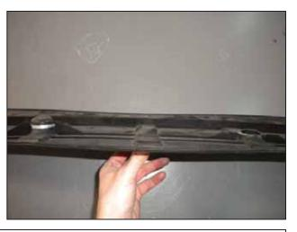
au. Two inner mounts and one reinforcement rib of the front under tray need some minor trimming.
