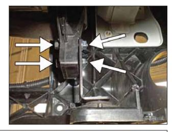
e. Install the radiator support brackets as shown using the M6 bolts removed in step 2aa and the supplied M6 nuts. Look for the "R" or "L" stamped on each bracket. The bolt should go through from the radiator side and the nut should be on the bracket side.
