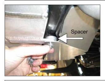
r. From underneath the car, install the short aluminum spacers on top of the intercooler mounting brackets. The spacers need to be between the intercooler brackets, and the cross member.
