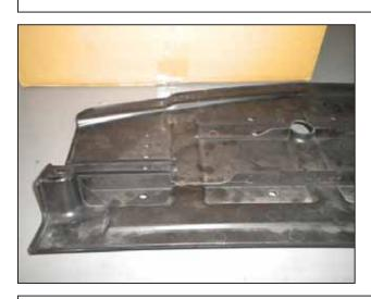
ax. Install the trimmed under tray using only the two outer mounts and two of the bolts removed in step 2(n). Check for clearance in the trimmed areas and modify if necessary.
