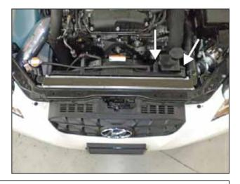
b. Remove the coolant reservoir by removing 2 self tapping screws and disconnecting the hose.
