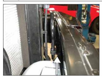
x. Install the bumper support, and check the alignment of the hole. The clip that holds the power steering cooler in place should snap into the hole. Readjust the M6 bolt/mount if needed.
