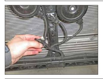
y. Unclip the ambient air temp sensor from the vertical support.
