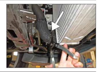
p. Use pliers to squeeze the spring clamp and slide it back on the charge pipe. Do this on both charge pipes.
