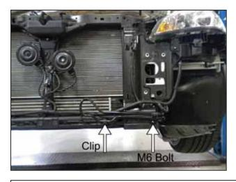
w. Unclip the plastic clip holding the power steering cooler in place. Also loosen the M6 bolt.
