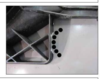
ak. After trimming, the fan shroud should look as shown.
