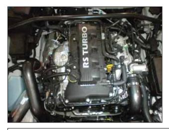
ah. Take some time to align the charge pipes for best fit. There should be about 1/4" minimum clearance between the pipes and other components in the engine bay.
