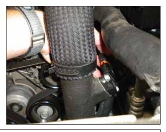
f. Unplug the boost pressure sensor located on the left charge pipe near the throttle body.
