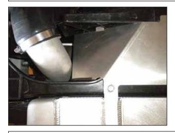
ap. Once the tabs are in position, secure the fan with the two M6 bolts removed in step 2(c). Plug in the fan and secure the wiring.
