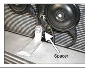
o. Install the long M6 bolt, one fender washer, and 1" tall spacer as shown. Let the bolt hang in place for now. Make sure that the ambient air temp sensor is rotated clockwise out of the way.
