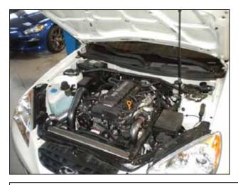
az. Make a final check for clearance between all components, and re-adjust if necessary. Be sure that all fasteners are tight including hose clamps and rubber mounts, and that the electric fan is plugged in before starting the vehicle.
