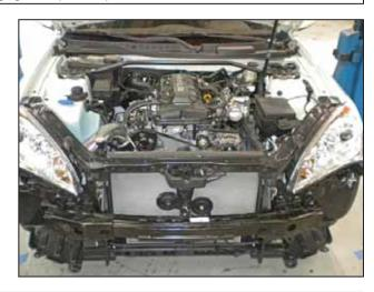
t. Remove the bumper cover and set it aside in a safe location.
