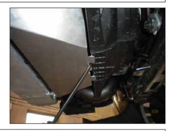
am. From under the car, manipulate the fan shroud and intercooler shroud so that the tabs snap into position.
