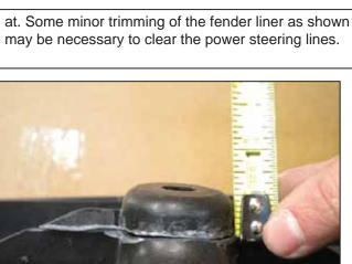
av. Mark the mounts as shown, and remove about  $\frac{1}{2}$ " from the mounts.
