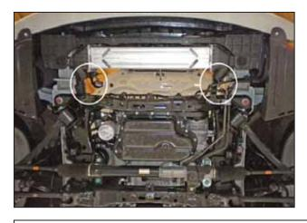
q. Slide the charge pipes off of the intercooler and remove them from the car.
