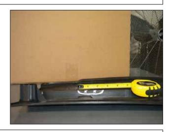
aw. Mark the reinforcement rib on the left side as shown, and trim.
