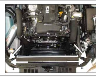
d. Remove the upper radiator mounts by removing 2 M6 bolts on each mount.
