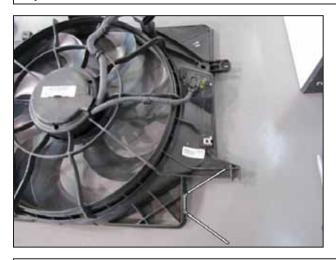
aj. On the right lower corner of the electric fan shroud, mark and trim the area shown for clearance with the charge pipe.
