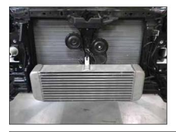
n. Once the right neck slips through the opening, lower the intercooler down all the way and tip the top towards the front so that both of the lower brackets are in place below the cross member.
