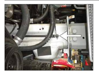
h. Move the ground wire to the lower bolt location and stack it on top of the existing terminal. Be sure the ground bolt is secure. Leave the top bolt hole vacant.
