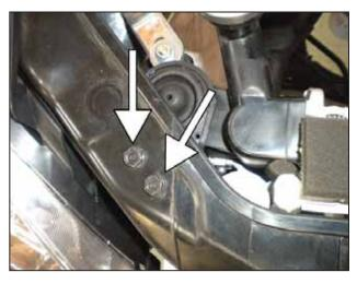
c. Reinstall both upper radiator brackets removed in step 2d.
