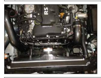
al. Lower the electric fan and shroud into place. Guide the lower tabs on the fan into the mounts on the radiator from underneath.
