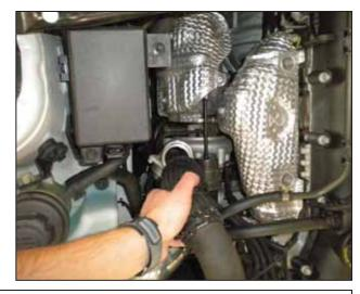
j. Pull the right charge pipe up and off of the compressor outlet.
