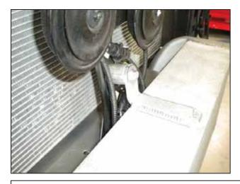
t. Run the top mounting bolt in and push the shroud toward the front of the car to reduce the gap between the intercooler and the shroud.
