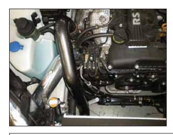
ad. Install the right charge pipe as shown. Line up the lower end of the pipe, and press the upper end down into the coupler on the compressor outlet. Secure it to the rubber mount with the supplied fender washer and M6 nut.
