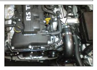
ag. Install one of the straight couplers onto the throttle body using 2 #44 clamps and install the left charge pipe as shown. Secure it to the rubber mount using the supplied fender washer and M6 nut. Plug in the boost sensor.
