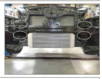
y. Attach the bumper support with the 6 M8 bolts and 2 M6 nuts removed in step 2(u).
