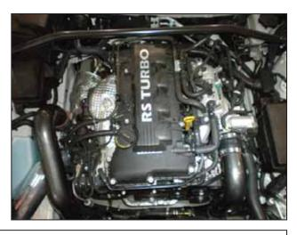
ai. Once proper fit is achieved. Tighten all hose clamps and rubber mounts.
