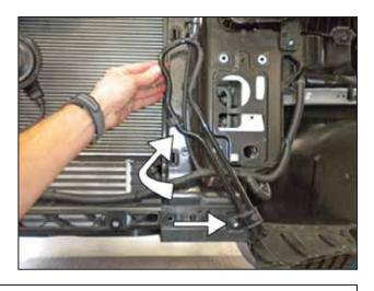
x. Rotate the power steering cooler as shown and retighten the M6 bolt to hold it in place temporarily.
