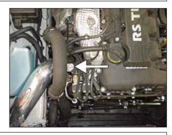
h. Remove the M8 bolt securing the right charge pipe to the bracket above the power steering pump.
