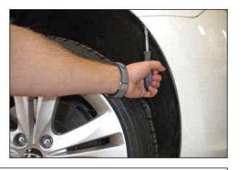
I. Remove one self tapping screw from each side of the bumper cover.
