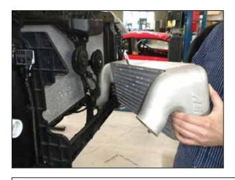
I. Inspect the end tanks of the intercooler and remove any packaging material that may obstruct the inlet and outlet. Begin the installation of the AEM® intercooler as shown. Guide the left intercooler neck into position, then lower the intercooler down, so that the left lower bracket slides under the cross member.
