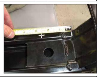
w. Measure 2.5" from the corner of the mount as shown. Mark and drill a 3/8" diameter hole. Debur and paint the edges of the hole to prevent rust.
