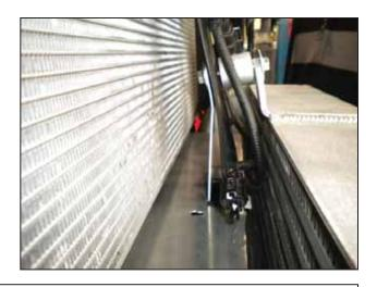
q. Install the shroud and attach it to the back of the bolt installed in step 3(o) using the supplied fender washer and M6 nut. Leave the nut loose for now. The tabs on the bottom of the shroud should rest below the tabs on the intercooler.
