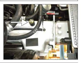
i. Install one of the supplied M6 rubber mounts into the vacant bolt hole from the previous step. Hand tighten the rubber mount.
