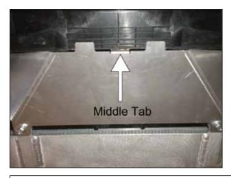
an. Push the bottom of the fan shroud toward the rear as shown to engage the bottom middle tab. The middle tab should rest on top of the fan shroud, and the two outer tabs should rest below the fan shroud.
