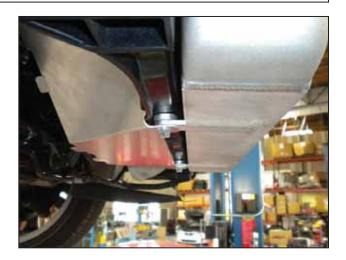
s. Attach the intercooler to the cross member with the supplied M6 bolts and washers. Lift up on the intercooler and run the bolts in, but do not tighten them all the way until everything is aligned.
