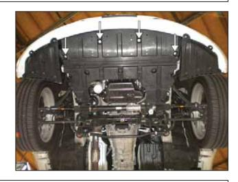
n. Remove the front under tray by removing 4 M6 bolts.
