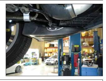
as. Check for clearance of the power steering cooler lines to the fender liner. Gently bend the lines and / or trim the fender liner as needed.
