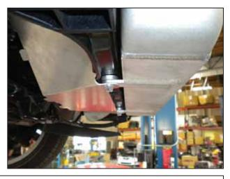
u. For best fit, push the intercooler toward the right side of the car. When the alignment of the shroud and the intercooler looks good tighten all three bolts.
