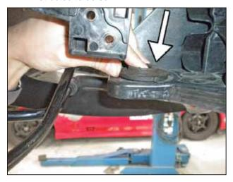
b. If the rubber grommets come out with the intercooler put them back in place.
