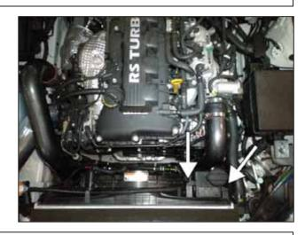
aq. Install the coolant reservoir using the two self tapping screws removed in step 2(b). Connect the overflow hose and ensure clearance between the reservoir and left charge pipe; readjust the pipe if necessary.
