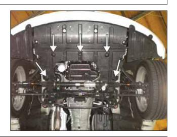
ay. Install the second under tray using the 5 M6 screws removed in step 2(o).
