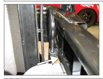
v. On the back of the bumper near the left mount, a hole needs to be drilled for mounting the power steering cooler.
