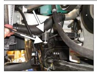
j. Install the other M6 rubber mount as shown with the small aluminum spacer under it. Hand tighten the rubber mount.
