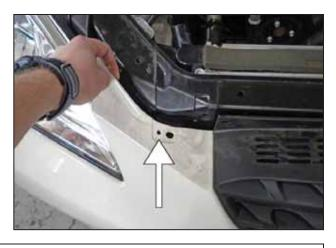
r. Lift up on the corners of the bumper cover to disengage the plastic pin on each side.
