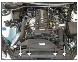
a. Remove the air scoop (if equipped) by removing the 4 clips.
