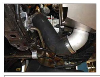
z. Install the lower coupler using two #44 clamps as shown.
