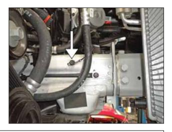
g. On the side of the left frame rail, locate the two M6 bolts used for attaching ground wires. Remove the ground wire from the top bolt location.
