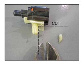
z. Use flush cuts to trim off the "key" on the clip so that the sensor can be rotated slightly. Then reinstall the sensor.
