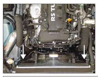
c. Remove the electric fan and shroud by removing 2 M6 bolts and unplugging the fan. Disconnect the plastic clip securing the fan wiring to the fan shroud.
