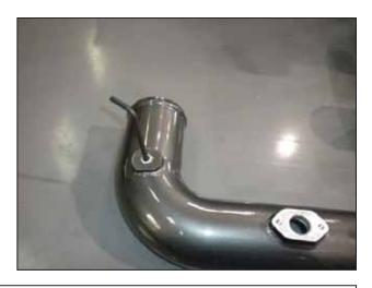
ae. If not using water injection, install the supplied 1/8" NPT plug into the water injection bung on the left charge pipe. Use some Teflon tape or thread sealant. If using an AEM® water injection system, install the injector using Teflon tape or sealant and follow the instructions provided with the water injection kit.
