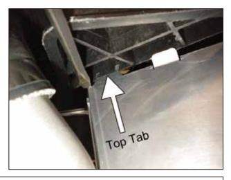
ao. Use a similar approach on each side of the intercooler shroud. The top tab should rest on top of the fan shroud and the lower tab should rest below it.
