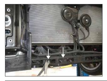
f. Using a pair of flush-cuts or similar tool, trim off the two plastic nubs on the front of the lower cross member.
