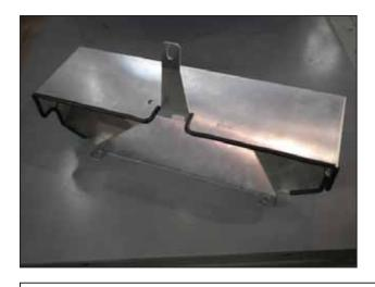
p. Install the supplied rubber edge trim on the intercooler shroud edges as shown. Cut and trim the rubber as needed.
