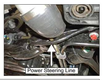
aa. Gently bend the power steering cooling line to clear the coupler. It is best to achieve at least 1/4" clearance between the power steering cooler line and the coupler. Take care to not kink the power steering lines.
