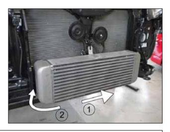
m. With the left neck in position, tip the top of the intercooler back and guide the right neck into position. The intercooler will have to be pushed all the way to the left side of the car for the right neck to slip past the opening.
