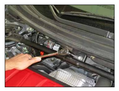
a. Using a 14mm socket, remove the (2) bolts holding the stock strut bar to the firewall bracket
