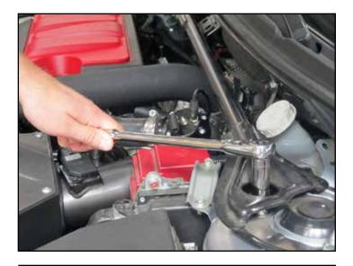
c. Remove the stock strut bar
