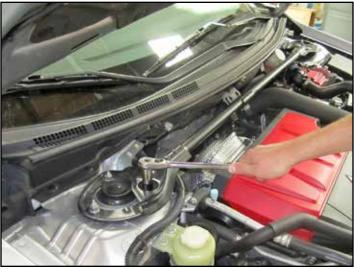
b. With the car on the ground, Use a 14mm socket to remove the (6) strut top nuts
