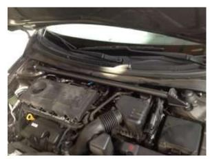
b. Place the AEM Strut Tower Bar over the strut top studs and washers, and replace the strut top nuts.
