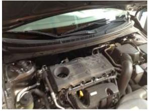
a. Remove the front and inside strut top nuts, that will be used to secure the AEM Strut Bar.
