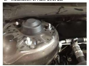
a. Place two (2) included washers over each of the strut top studs, as shown.
