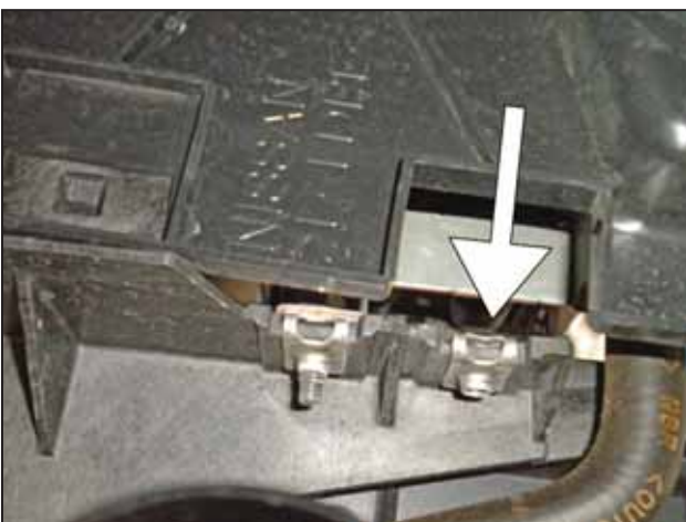
ay. Locate the lower windshield washer reservoir clip on the passenger side fender shroud.
