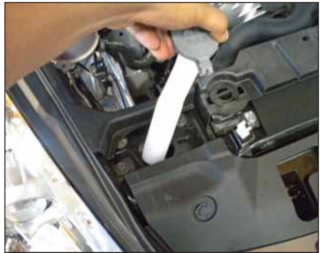
ap. Remove the windshield washer fluid spout.
