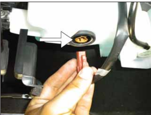
o. Disconnect the brown connector connected to the windshield washer reservoir level sensor.
