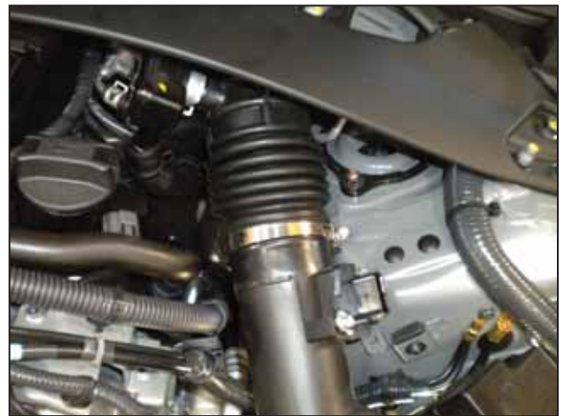
ab. Loosen the hose clamp connecting the driver side inlet tube to the airbox.
