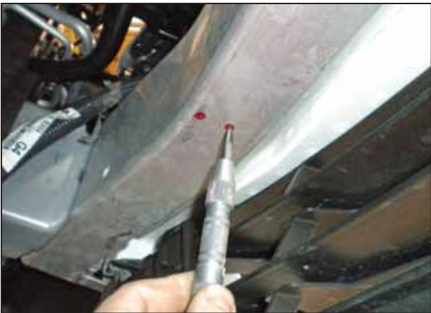
af. Remove the bracket, use a center punch to mark the four locations that are marked for drilling.
