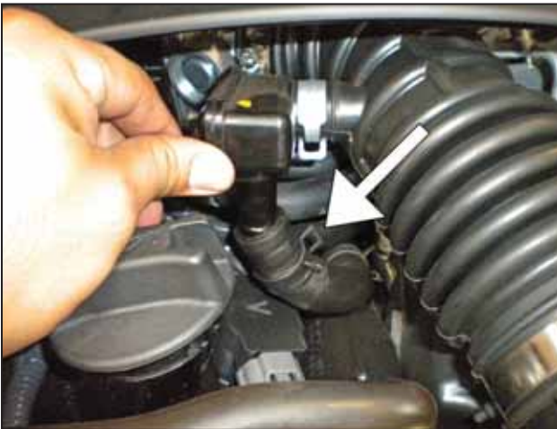
ae. Release the hose clamp to remove the PCV hose.
