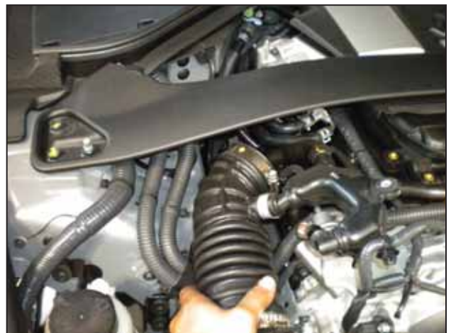
an. Remove the passenger side inlet tube.
