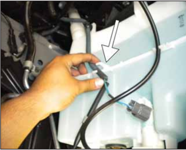
q. Unhook the wire harness from the windshield washer reservoir.
