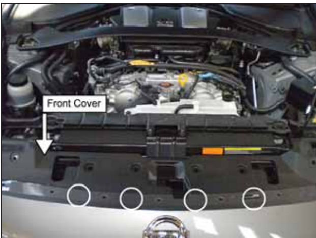
as. Remove the front black cover by lifting up on the inner edge of the cover (just below the black plastic trim) to avoid breaking the 4 plastic prongs inserted in the support bracket. The circled areas specify the approximate locations of where the prongs attach to the support bracket.
