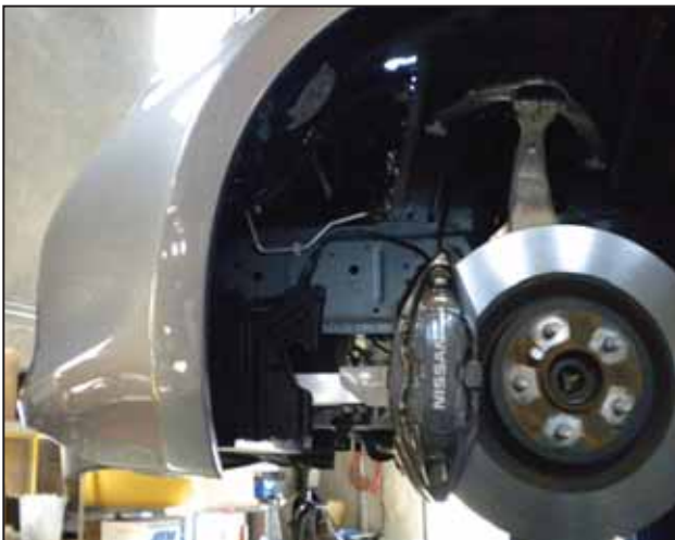
i. Remove the driver side fender liner.
