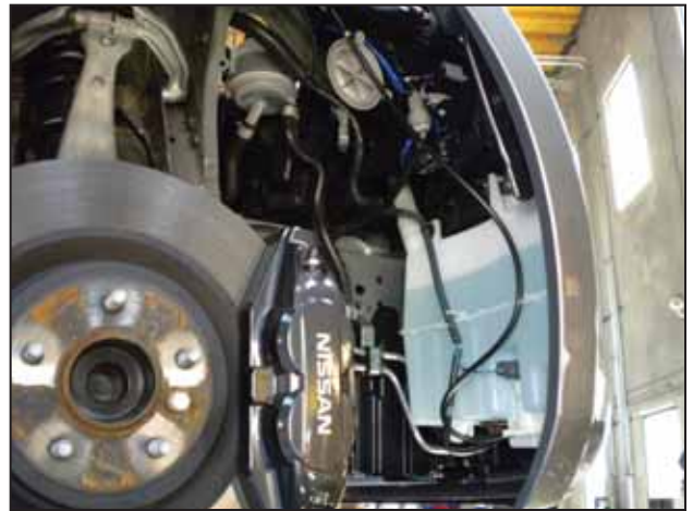
n. Remove the passenger side fender liner.
