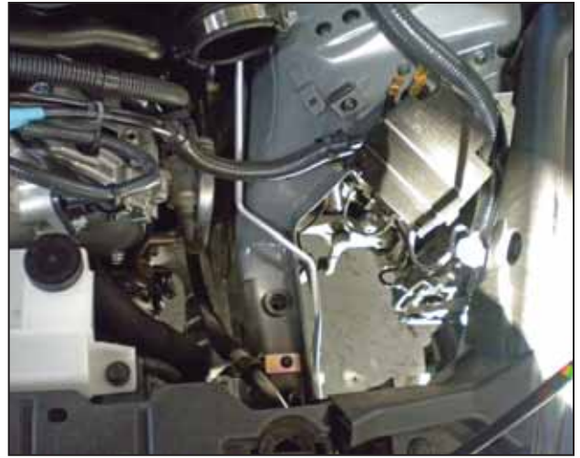
ad. Remove the driver side airbox.
