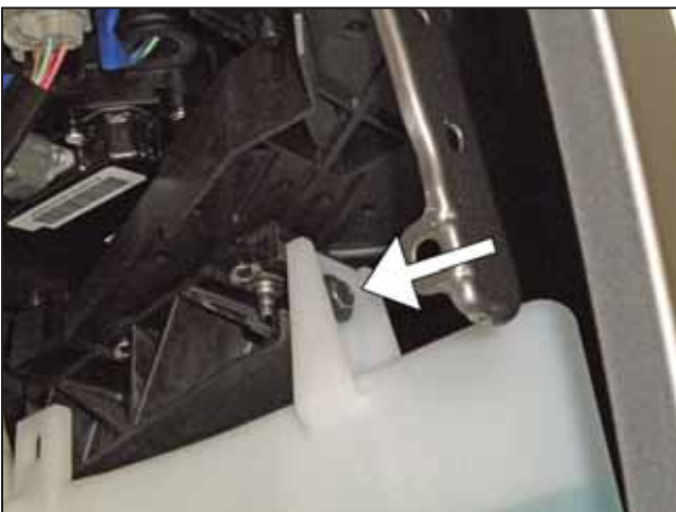
u. Remove the upper bolt securing the windshield washer reservoir to the vehicle.
