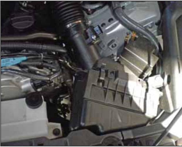
ac. Disconnect the inlet tube from the driver side airbox.
