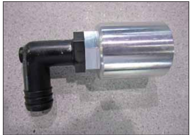
ao. Screw the 90° fitting into the filler neck adapter. Use some Teflon tape, or thread sealant on the threads to prevent leaks.
