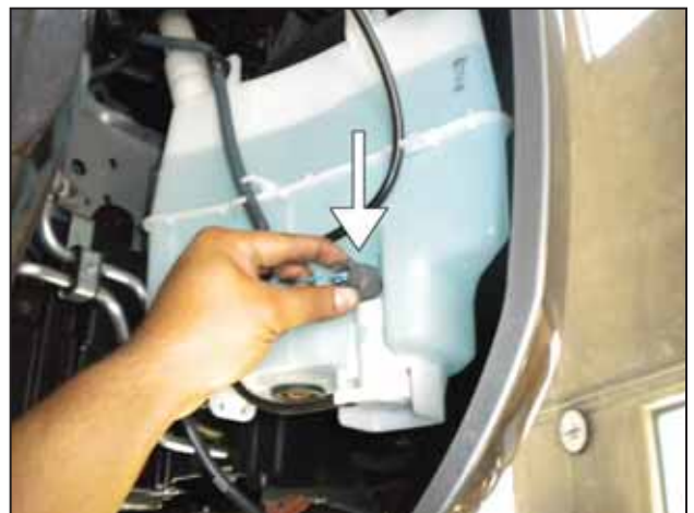
p. Disconnect the grey connector connected to the windshield washer reservoir pump.
