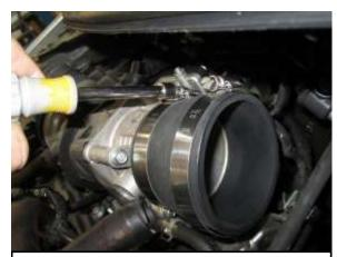
C. Tighten the (#24) hose clamp on the throttle body end.
