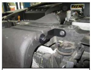
Z. Secure the air inlet scoop's bracket to the radiator support using one M6 bolt (#15).
