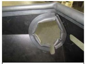
I. Install the rubber edge trim (#16 and 17) around the intake tube opening in the heat shield (#11).
