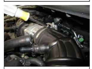
J. Loosen the hose clamp that secures the Inlet tube to the throttle body.
