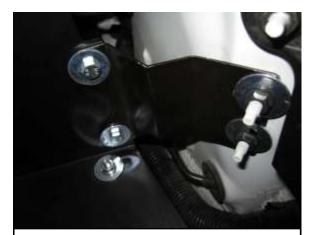
O. Align the heat shield's bracket with the two studs, secure in place using two washers (#5) and the two OEM nuts removed in step 2 S
