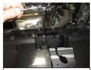
N. Remove the 6MM bolt on the top grill support.
