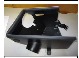
K. Install the rubber edge trim (#12) onto the top edge of the heat shield.
