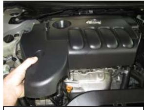
B. Lift up on the bottom of the engine cover and remove it from the vehicle.
