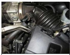
H. Release the two clips securing the MAF sensor harness to the air box.
