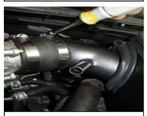
AG. Align the intake pipe with the throttle body's coupler and secure the (#22) hose clamp.
