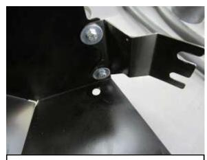
I. Attach the provided bracket (#14) onto the heat shield using two M6 bolts (#7) and two washers (#5).
