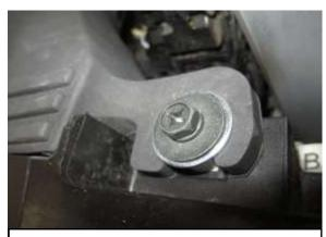
V. Secure the air inlet hose using the OEM bolt and washer (#5) as shown.
