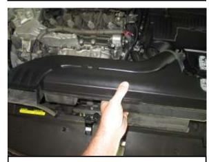
D. Remove the stock intake scoop from the vehicle.
