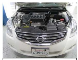
AM. Re-install the grill using the factory clips removed in step M.
