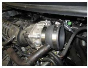
B. Install coupler (#23) onto the throttle body and mount the (#22) and (#24) hose clamps as shown.
