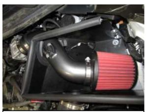
AF. Mount the AEM air filter (#20) onto the intake tube and secure using a (#22) hose clamp.
