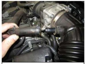
F. Remove the hose from the valve cover vent.
