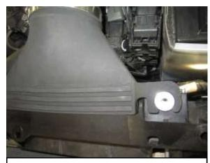
U. Install the mounting block (#9) onto the air inlet hose as shown.
