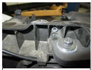
AA. Secure the M6 bolt installed in the previous step by attaching one M6 nut (#4) to the end of the bolt that passed through the radiator support.
