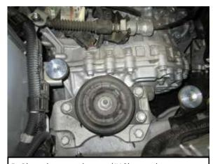
D. Place the two adapters (#10) onto the factory rubber grommets as shown.
