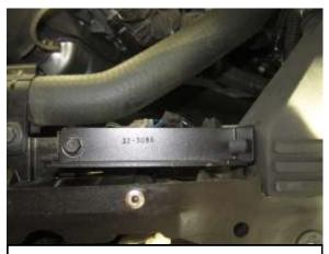
T. Attach bracket (#13) to the air inlet hose and to the radiator support using the provided M6 bolt (#15).
