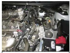
L. Remove the factory air box system from the vehicle.
