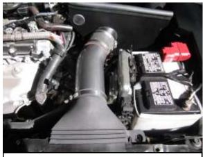
S. Install the air inlet hose assembly into the engine bay as shown.
