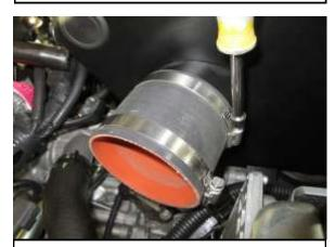
Q. Install the 3.5" coupler (#2) with two #3 hose clamps onto the heat shields inlet, tighten the hose clamp on the heat shield inlet end.
