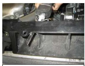
T. Cut the radiator support to make room for the AEM front scoop.
