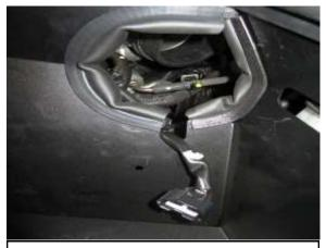
AD. Feed the MAF sensor wire harness into the inside area of the heat shield as shown.
