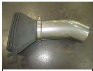
R. Attach the air inlet hose (#8) to the air intake tube (#6) and loosely secure with a (#3) hose clamp.
