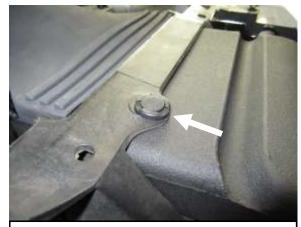
Y. Install the OEM clip as shown.
