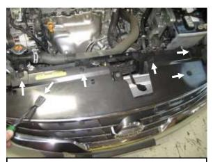
M. Remove the six clips on the top of the front grill.
