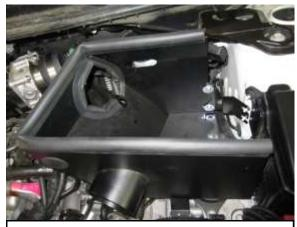
M. Place the heat shield in the vehicle's engine bay, ensuring the threaded ends of the bolts from step G align with the openings on the bottom side of the heat shield.
