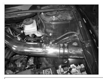
k. Align the upper intake tube with the lower intake tube and slide the coupler over the upper intake tube so that the coupler covers both tubes evenly. Loosely secure the three #48 hose clamps.
