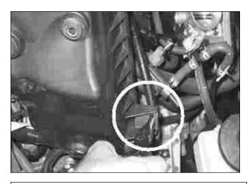
I. Tilt the air filter housing up towards the engine and use needle-nose pliers to unclip the MAF sensor/ VSV wire harness from the housing.
