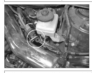
m. Use the screw removed in 2e to secure the VSV and harness bracket (7-7717) to the bracket on the upper intake pipe. Reconnect the short vacuum line.
