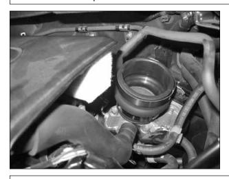
h. Install the small end of the hump hose (5-574) onto the throttle body and secure with #40 hose clamp. Install a #48 hose clamp loosely over the large end of the hump hose.
