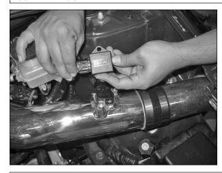
o. Connect the female connector coming from the vehicle to the male connector located on the ETI module.
