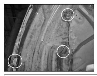
q. Remove the screw and clips holding on the driver side fender liner.
