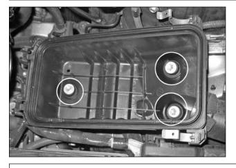
j. Remove the 3 bolts holding the air box in place.
