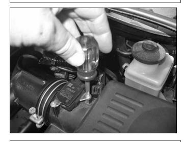
c. Remove the mass airflow sensor from the intake tube (Be sure to keep in a safe place to be used later.).
