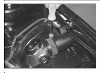
m. Remove the upper clip securing the lower intake tube.
