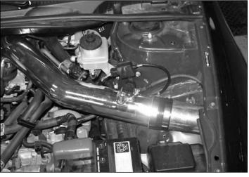
AEM® intake system installed
