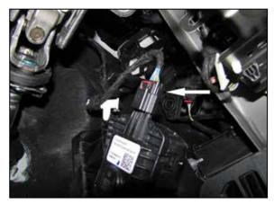
1. Locate the pedal wiring harness connection on top of the throttle pedal assembly and release the red locking tab and disconnect the electrical connection.
