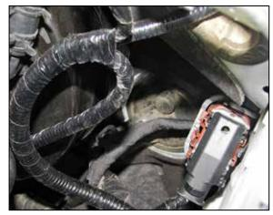
6. Create a small hole in the fire wall grommet and route the pedal harness through the hole into the engine compartment.
