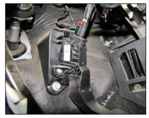
4. Locate the throttle pedal connector under the instrument panel. Release the red locking tab and disconnect the connector from the pedal assembly.
