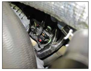
3. Connect the provided Boost module wiring harness to the factory harness and to the fuel pressure sensor. Route the harness to the driver side inner fender.
