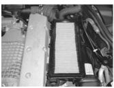
8. Install the K&N FILTERCHARGER® air filter into the airbox
