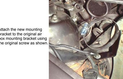
Attach the new mounting bracket to the original air box mounting bracket using the original screw as shown.
