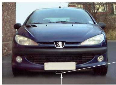
**1.** Attach the new rubber cold air scoop to the front lower spoiler trim by piercing / drilling two 3mm holes in the trim and securing the scoop with 2 small plastic ties.
