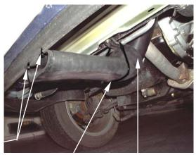
**2.** Secure the rear of the scoop to the front lower cross member using a long plastic tie.
