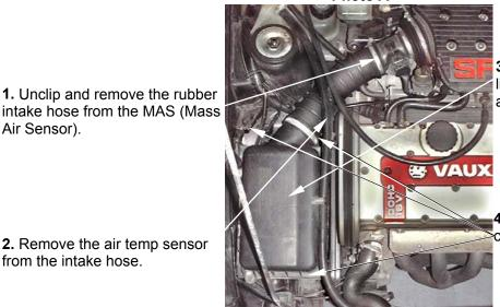
**3.** Unclip and remove the air box lid assembly from the air box base and remove from the car.
