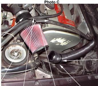
**3.** Fit the air temp sensor into the hole in the side of the filter neck.
