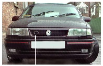
Feed the flexi cold air hose to the front grille, then feed a plastic tie through the hole in the end of the hose and secure the hose to the grille. (It may be necessary to remove the grille to aid the fitment of the hose).
