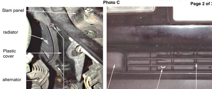
1. Remove the 2 securing screws which secure the plastic cover panel to the side of the radiator.
