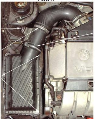
**4.** Unscrew and remove the MAS from the air box lid.
