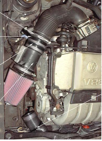
5. Fit the new filter onto the MAS. Do not push in beyond the step as this will affect air flow. Tighten the clip until the filter just turns, Rotate the filter until the K&N logo is straight then tighten the clip one full turn (360 degrees) no more, <u>Do not</u> overtighten the clip.
