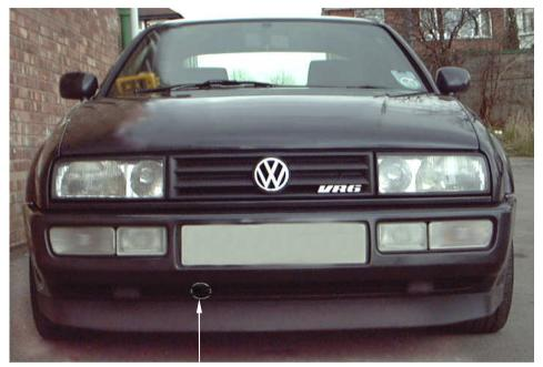
Pierce a 3mm hole in the end of the flexi cold air hose and feed the hose down to the lower grille. Secure the hose to the lower grille using a long plastic tie, ensure the hose is in the air stream.
