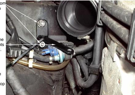
**1.** Remove the nuts from the 2 studs located on the suspension turret.
