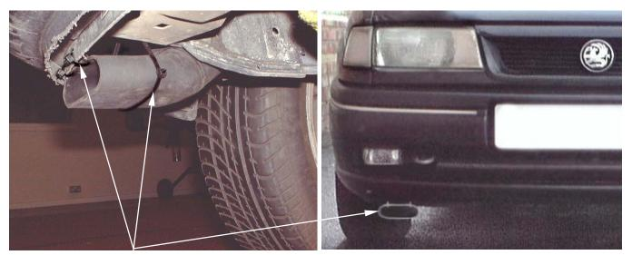
Pierce / drill two 3mm holes in the front bumper trim, secure the new cold air scoop to the front bumper using 2 plastic ties. Insert the flexi cold air hose into the new scoop, secure the scoop to a hole in the cross member with a long plastic tie.
