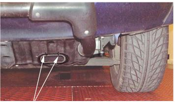
2. Insert the flexi cold air hose in the rubber scoop, then refit the undertray to the vehicle. Insert the rubber scoop into the pre cut hole in the undertray. Pierce / drill two 3mm holes in the undertray and secure the scoop to the undertray using 2 medium plastic ties supplied. (Ensure the scoop is horizontal to the floor and not angled downwards as this will affect air flow in the scoop.).
