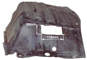
1. Taking all of the necessary safety precautions as per the manufacturers instructions, raise the front of the car. Unscrew and remove the L.H.S. undertray. Again taking all of the necessary safety precautions cut a rectangular hole in the undertray using the position and dimensions illustrated. Line the edge of the hole with the seal clip supplied (It may be necessary to trim the clip to suit the circumference of the hole)
