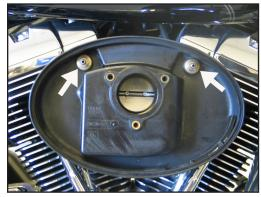
5. Remove the two breather / air filter base mounting bolts shown.
