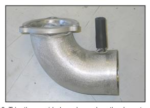
8. Trim the provided crankcase breather hose to a length of 1.5" and then install it onto the K&N $^{\odot}$  intake tube as shown.
