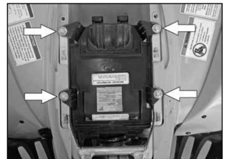
8. Remove the four bolts securing the air box to the frame.
