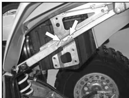
5. Remove the four bolts which secure the air box mounting bracket to the frame and then remove the brackets, there are two bolts holding each bracket.
