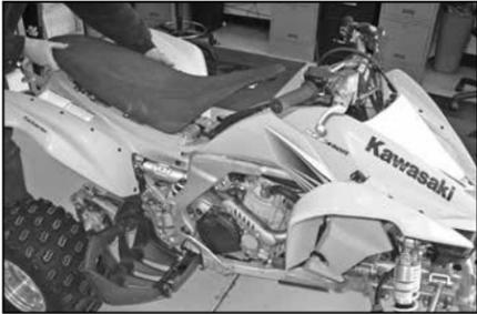
2. Unlock the seat and remove it from the vehicle.
