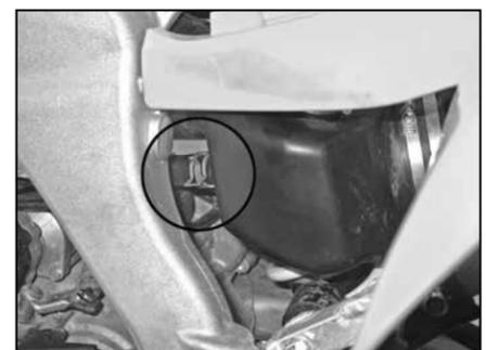
10. Release the spring clamp securing the crank case vent line to the intake resonator chamber and then disconnect the crank case vent line.
