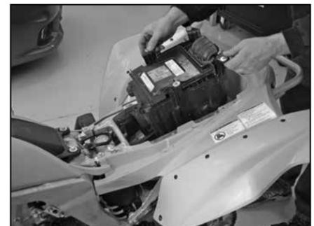
9. Remove the factory air box from the vehicle.
