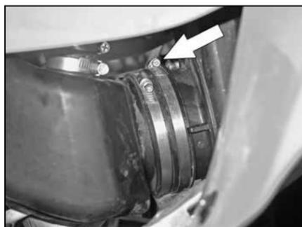
7. Loosen the hose clamp which secures the stock intake tube to the factory air box.
