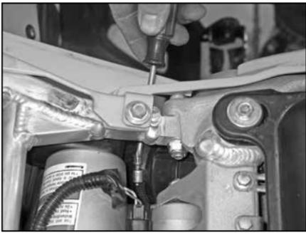
11. Loosen the hose clamp which secures the intake resonator to the stock intake hose.
