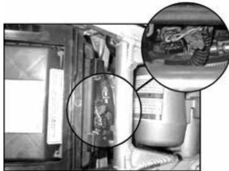
6. Remove the screw which secures the inlet air temperature sensor to the air box. Then remove the air temperature sensor from the air box.
