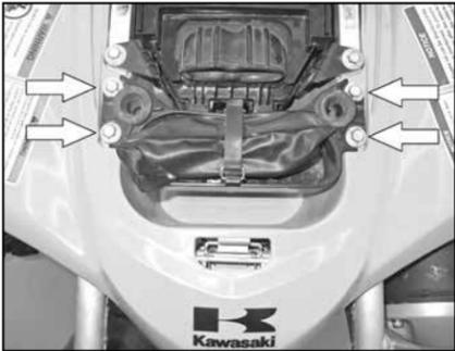
3. Remove the four bolts which secure the tool tray. Then remove the tool tray from the vehicle.
