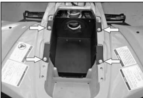
14. Install the K&N® air box into the chassis and secure with the factory air box mounting bolts.
