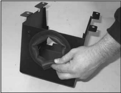
13. Install the provided edge trim into the heat shield as shown.
