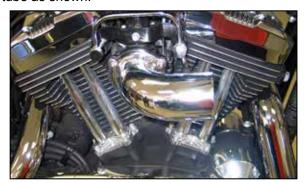
10. Install the K&N® intake tube onto the throttle body while attaching the vent hose to the vent tube and secure with the provided hardware.
