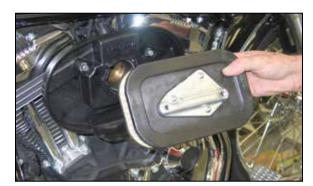
4. Remove the air filter as shown.
