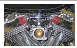
7. Install the K&N® crankcase breather tube onto the vehicle using the provided hardware. NOTE: Do not completely tighten the breather bolts at this time.
