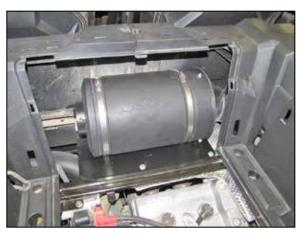
17. Install the filter canister assembly onto the mounting tray and connect the fresh air inlet hose. Adjust the canister and hose for best fit and then secure the canister and hose with the hose clamps. NOTE: Due to differences in the production factory foil heat shield, the heat shield may need to be reformed to allow the canister and fresh air hose to fit together.
