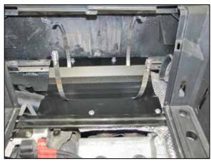
11. Install the filter base plate assembly as shown using the provided hardware.
