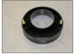
13. Install the two provided 6mm studs into the radius filter adapter as shown. **NOTE: Be sure to add a drop of the provided**
