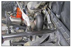
19. Install the K&N<sup>®</sup> intake tube into the coupler hose and secure with the provided hose clamp. Connect the waste gate vacuum hose to the vacuum switch and secure with the provided tie wrap.
