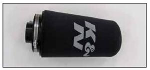
20a. Install the provided foam wrap onto the  $K\&N^{\mbox{\scriptsize \$}}$  air filter.
