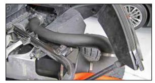
29. Install the K&N<sup>®</sup> fresh air intake tube assembly and 90° coupler hose (08502) to the fresh air tube mount and air filter housing, adjust for best fit and then secure with the provided hose clamps.
