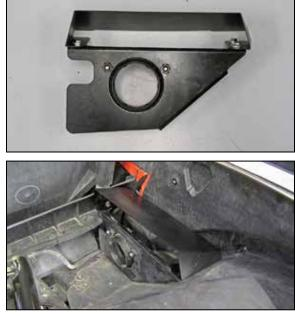
13. Install the fresh air scoop onto the tube mount using the provided hardware, then reinstall the assembly to the body using the factory bolts from the previous step.
