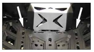
2. Remove the two bolts and nuts shown that secure the cargo tray to the frame. **NOTE: The nuts are on the underside and will need to be held with a wrench while loosening the bolts.**
