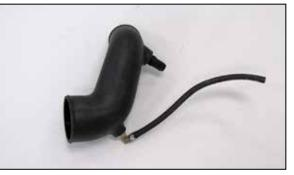
16. Install the waste gate hose and fitting along with the provided crank case vent hose fitting into the K&N $^{\circ}$  intake tube as shown.
