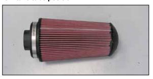
20. Install the provided filter adapter into the K&N<sup>®</sup> air filter and secure with the provided hose clamp.
