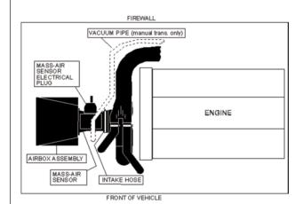
**TWIN-TURBO ENGINE COMPARTMENT**
