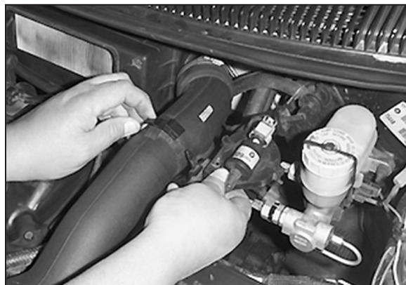
4. Detach the hose clip from the intake tube.
