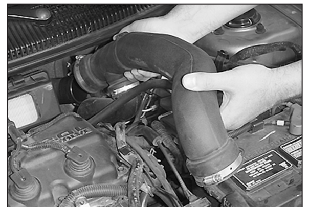
8. Remove the intake tube.
