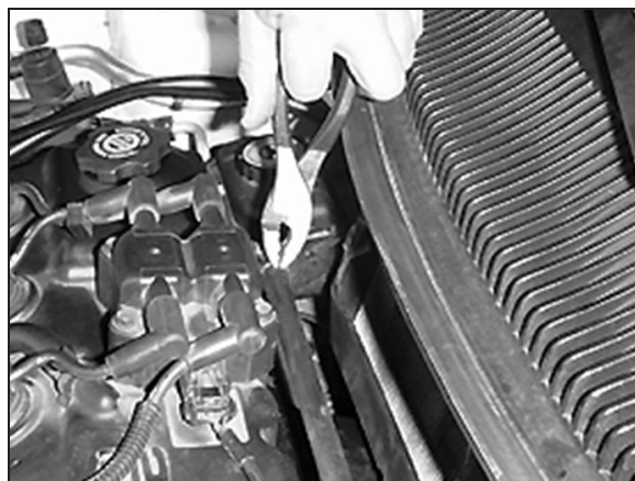
5. Disconnect the PCV line from the fitting on the valve cover.
