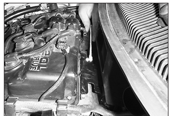
9. Loosen and remove the two bolts that retain the airbox mounting bracket. Note: These bolts will be reused
