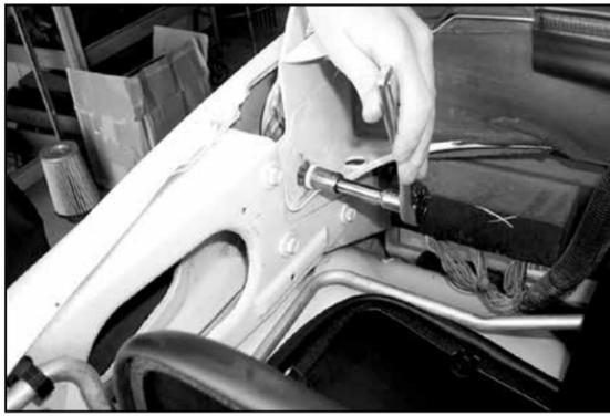
15. Loosen and remove the bolt that retains the hood hinge to the inner fender and remove hood hinge bolt from vehicle.
