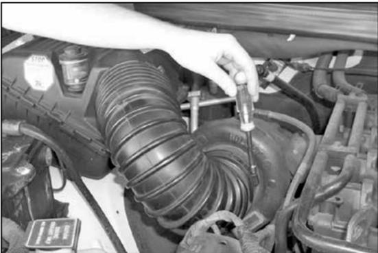
2. Loosen the hose clamp on the stock intake tube at the turbo.
