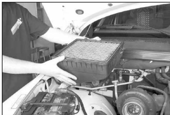
4. Pull upward firmly on the airbox base to release it from its mounting studs and remove.
