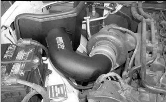
11. Slide the K&N® intake tube through the heat shield and attach the hump hose to the flange on the turbo.
