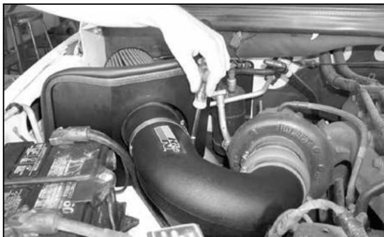
19. Attach saddle bracket to the intake tube with hose clamp provided. Adjust the bracket to achieve appropriate clearance for intake tube and tighten hardware.
