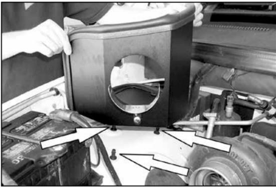
10. Install heat shield onto the locating studs as shown above.
