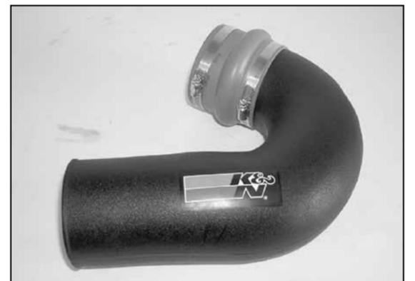
9. Attach the hump hose onto the K&N® intake tube as shown.
