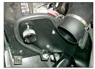
24. Install the K&N® air filter onto the air temperature sensor as shown.
