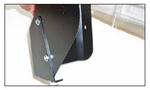
8. Install the large "L" bracket onto the heat shield with the provided hardware.
