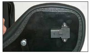
12. Install the temperature sensor onto the heat shield with the provided hardware as shown.
