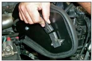
15. Reconnect the air temperature sensor electrical connection as shown.
