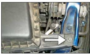
5. Loosen and remove the 10mm nut that retains the air box to the vehicle.
