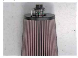
23. Install the grommet and air filter minder that was removed in step 21 onto the K&N® air filter as shown.
