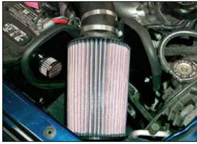
25. Install the K&N® air filter onto the intake tube as shown.
