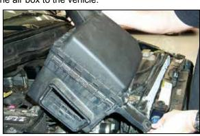
6. Remove the complete air box assembly from the vehicle as shown.
