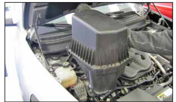
5. Lift up the air filter housing to dislodge it from the mounting grommets and then remove the complete air filter housing assembly from the vehicle.
