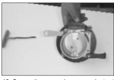
12. Secure the mass air sensor adaptor to the mass air sensor using the rubber gasket and hardware provided, with brackets positioned as shown.
