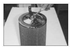
15. Using the hardware provided, install and secure the bracket onto the end of the Filtercharger element.
