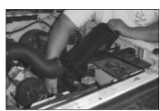
8. Disconnect the air inlet from the airbox base and remove the airbox base.
