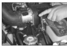
14. Install the mass air sensor into the intake tube and slide bracket over stud, then secure with nut that was removed in previous step.
