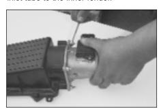
11. Using a 10mm wrench, loosen and remove the four nuts that hold the mass air sensor to the airbox lid.
