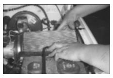
16. Install the Filtercharger element onto the mass air sensor adaptor.
