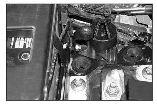
9. Install the "L" Bracket onto the existing air boxmounting tray, with supplied 8mm nylock nut.
