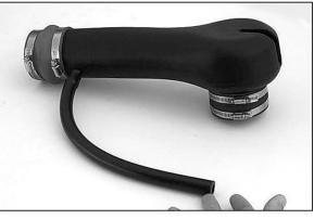
16. Install the silicone vent hose onto the new intake tube as shown.
