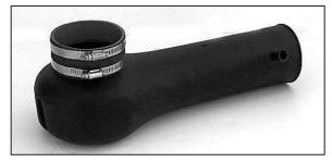
14. Install the silicone hose onto the new intake tube.
