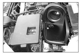
13. Install the heat shield assembly onto the vehicle as shown.
