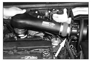
17. Install the new intake tube onto the mass air sensor.
