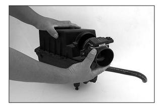
7. Unscrew the mass air sensor from the air box then remove the mass air sensor.
