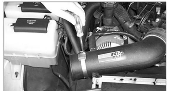
19. Re-install the K&N intake tube onto the throttle body then secure the intake tube to the saddle bracket assembly with the provided hose clamp.
