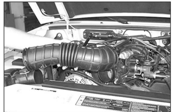
6. Loosen the hose clamp at the throttle body and at the mass air sensor, then remove the stock air intake tube as shown.
