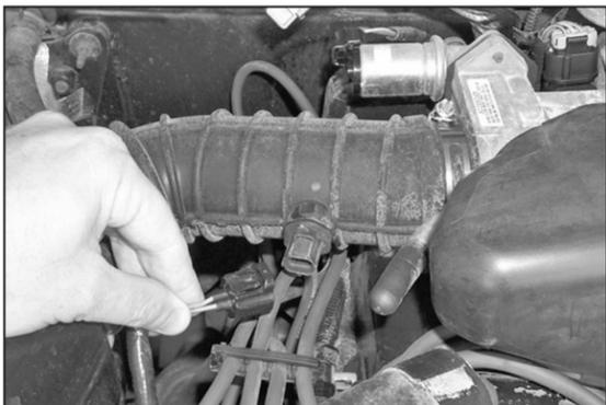
2. Disconnect the air temp. electrical sensor as shown.
