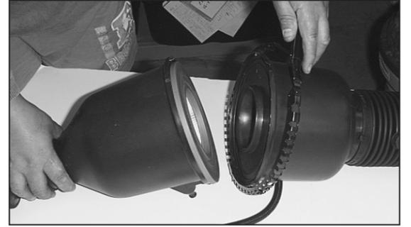
23. Open the air cleaner assembly and isolate the mass air sensor assembly.
