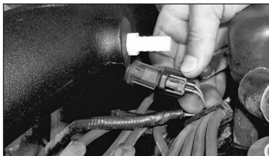
20. Reconnect the air temp. electrical connection as shown.
