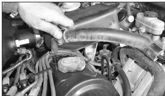
21. Remove the crank case vent hose from the valve cover as shown.
