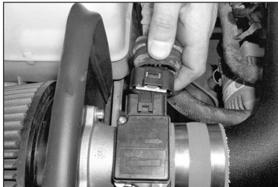
33. Reconnect the mass air electrical sensor as shown.
