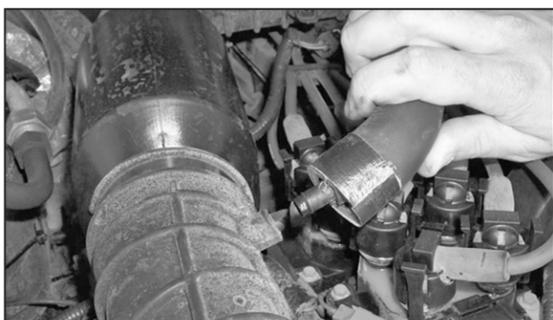
3. Remove the crank case vent from the intake tube as shown.
