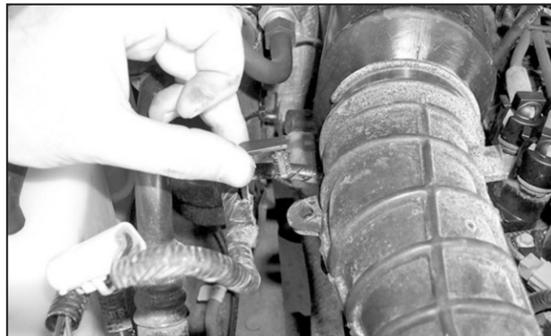
5. Disconnect the mass air wiring loom from the intake tube as shown.
