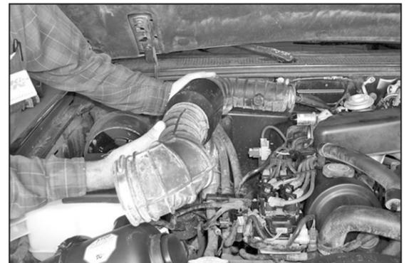
7. Remove the intake tube as shown.
