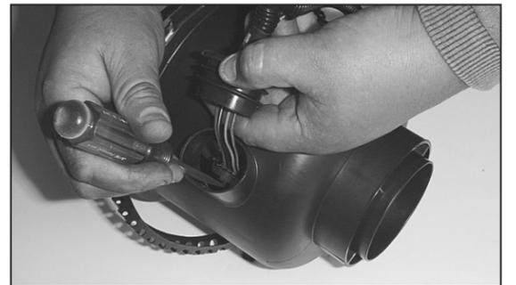
24. Slide the rubber grommet back and disconnect the primary mass air sensor electrical connection, using a flat blade screwdriver.
