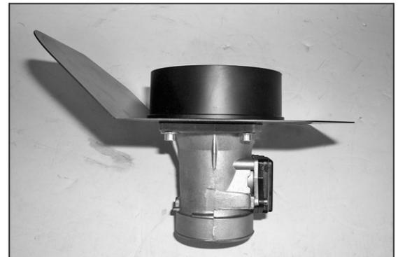
27. Assemble the heat shield and filter adapter onto the mass air sensor with the provided hardware.
