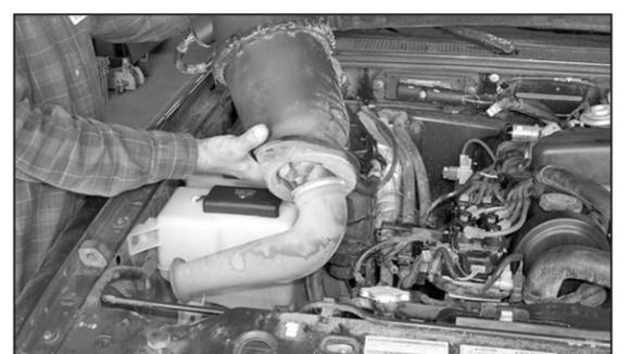
9. Pull firmly up on the air box to remove from vehicle.
