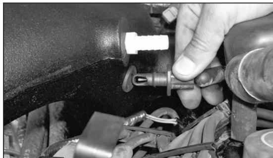
19. Install the air temp. sensor into the new K&N intake tube as shown.
