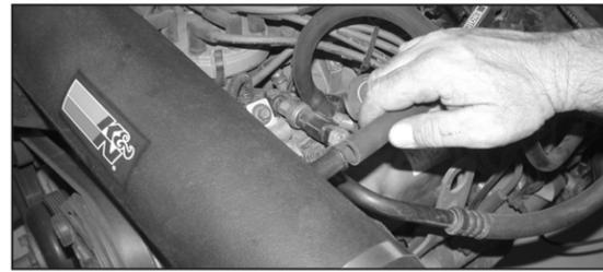
16. Remove the crank case vent tube from valve cover then connect the provided silicone hose to the valve cover, then connect to the intake tube as shown. Trim hose for best fit.
