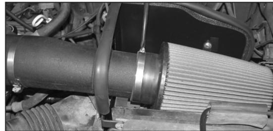
17. Install the air filter onto the new intake tube as shown.
