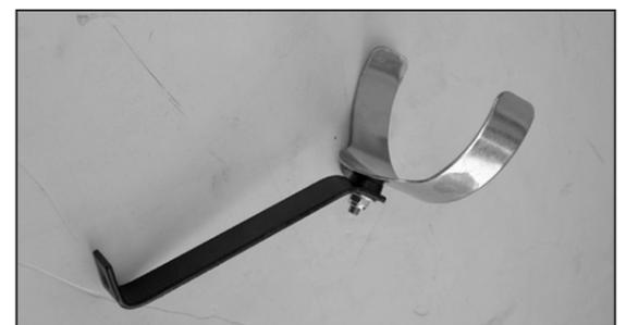
6. On vehicles that come equipped with A/C, assemble the saddle bracket onto bracket (07164) as shown.
