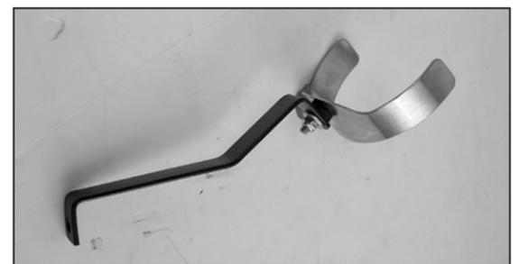
6a. On vehicles that do not come equipped with A/C, assemble the saddle bracket onto bracket (07165) as shown.
