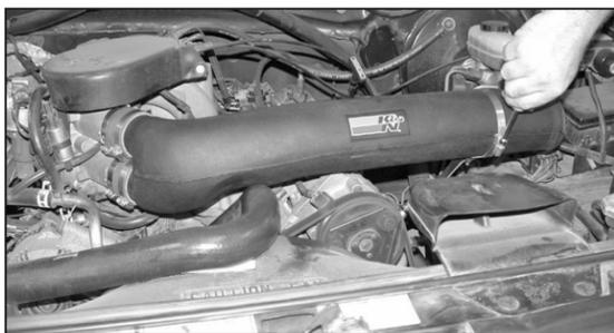
15. Install the new K&N® intake tube onto the throttle body, then secure the intake tube to the saddle bracket as shown.
