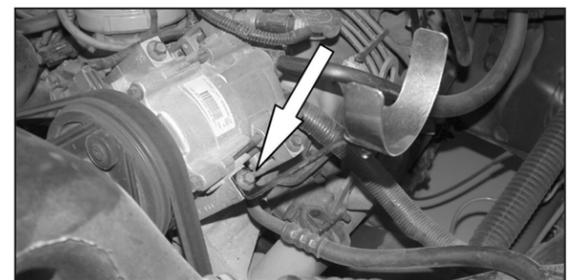
7. On vehicles that come equipped with A/C, remove the front lower A/C mounting bolt. Then secure the saddle bracket assembly from step 6 onto vehicle as shown.
