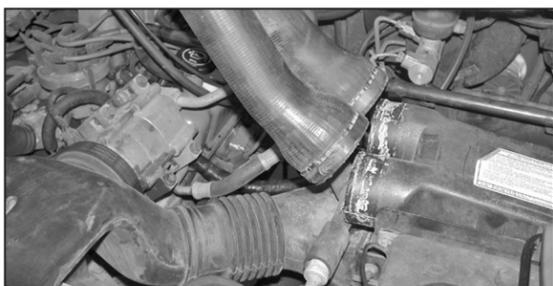
3. Loosen the two hose clamps at the airbox then remove the two intake tubes from the air box as shown.
