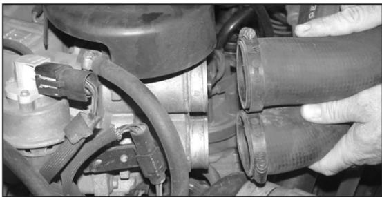
2. Loosen the two hose clamps at the throttle body, then remove the two intake tubes from the throttle body as shown.
