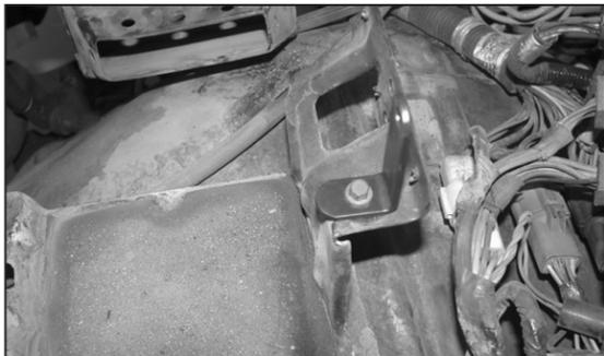
10. Install the provided bracket (07879) onto the air box mounting bracket as shown using one of the bolts that was removed in step 5.
